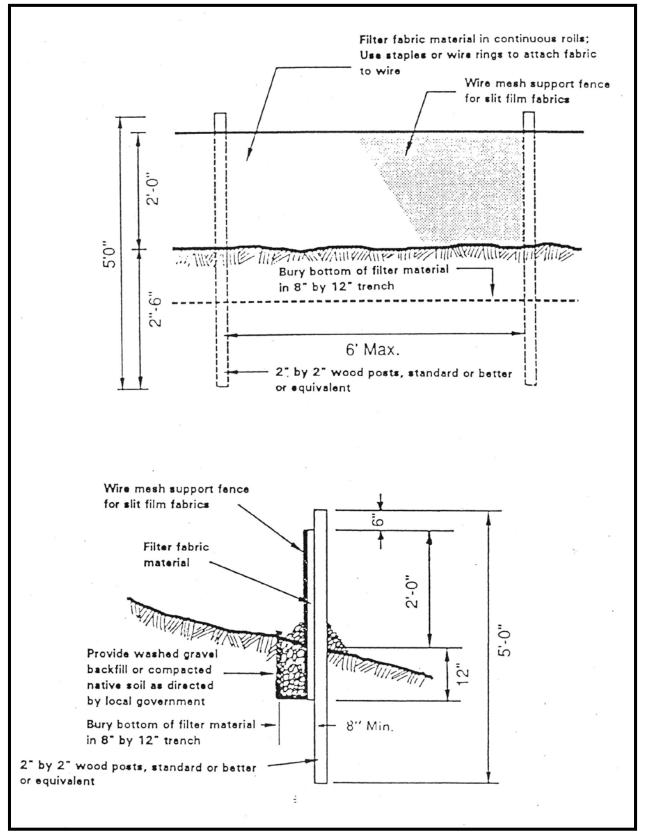
Figure 14. Silt Fence Details.
