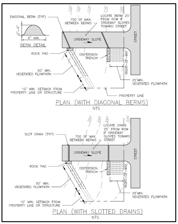
Figure 5.6. Typical Concentrated Flow Dispersion for Steep Driveways.
