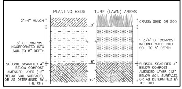
Figure 5.1. Cross-section of Soil Amendment.
