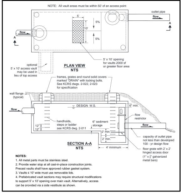
Figure 5.22. Typical Detention Vault.
