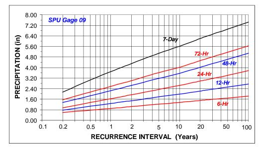
Figure 10. Precipitation-Magnitude-Frequency Estimates for SPU Gauge 09.
