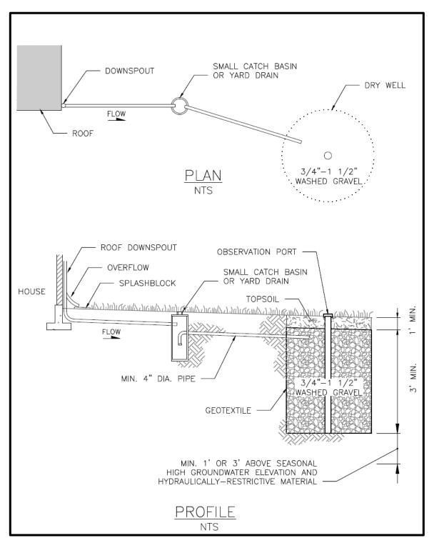
Figure 5.9. Typical Infiltration Drywell.
