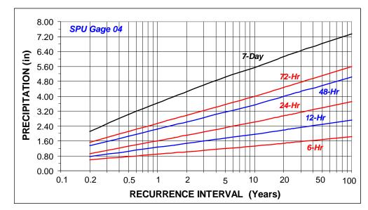
Figure 6. Precipitation-Magnitude-Frequency Estimates for SPU Gauge 04.
