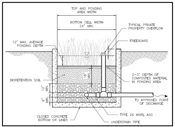
Figure 5.25. Non-infiltrating Bioretention Facility with Vertical Sides.
