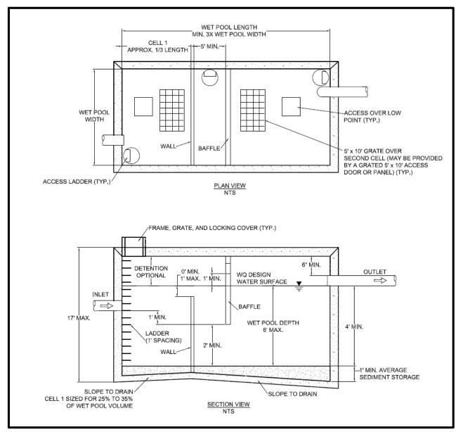
Figure 5.27. Typical Wet Vault.
