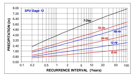
Figure 13. Precipitation-Magnitude-Frequency Estimates for SPU Gauge 12.
