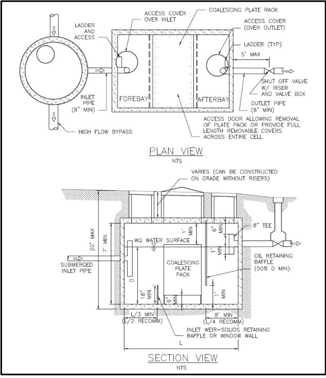
Figure 5.29. Typical Coalescing Plate Separator.
