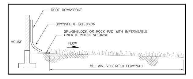
Figure 5.2. Typical Downspout Splashblock Dispersion.
