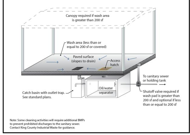
Figure 4. Schematic of Wash Pad with Sump.
