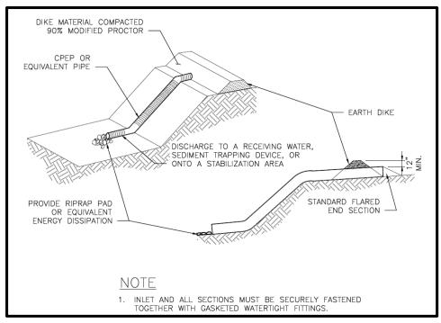
Figure E.7. Pipe Slope Drain Details.
