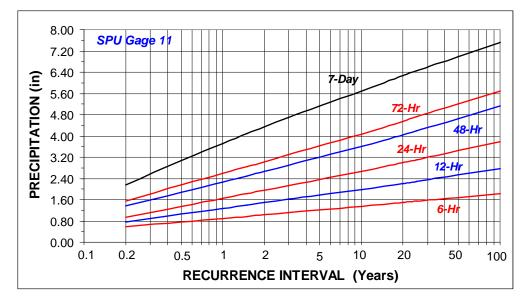
Figure 12. Precipitation-Magnitude-Frequency Estimates for SPU Gauge 11.
