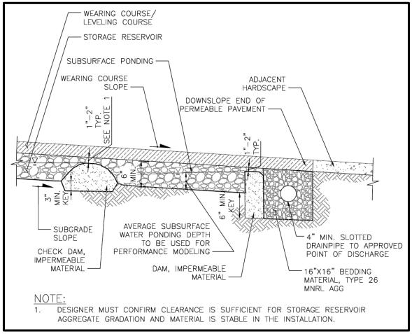
Figure 5.16. Typical Permeable Pavement Facility with Checkdams.
