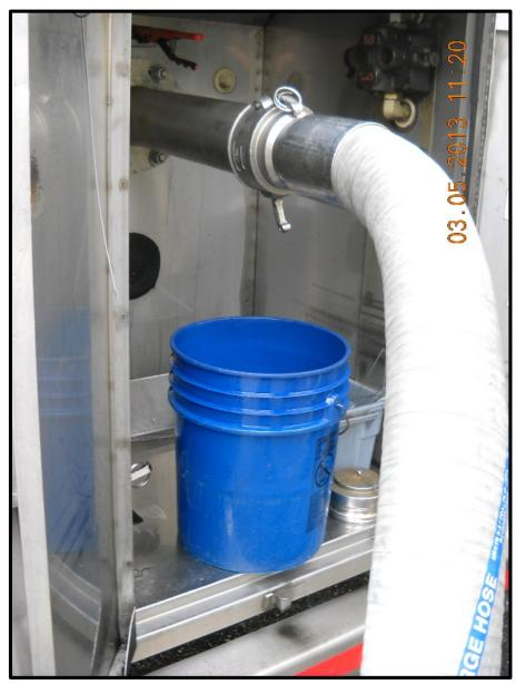
Figure 5. Temporary Containment Device Placed Under a Hose Connection.
