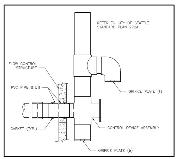
Figure E.1. Simple Orifice.
