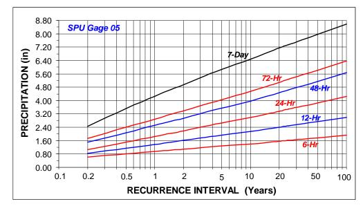
Figure 7. Precipitation-Magnitude-Frequency Estimates for SPU Gauge 05.
