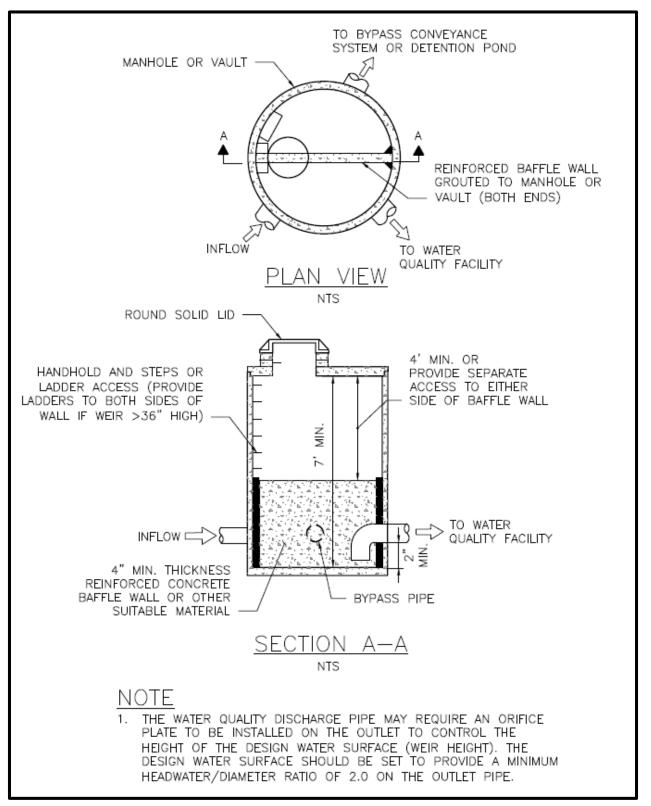
Figure E.4. Flow Splitter Example A.
