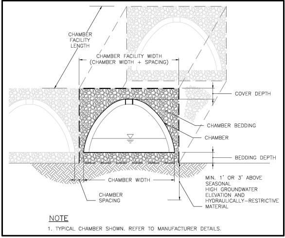
Figure 5.18. Typical Infiltration Chamber.
