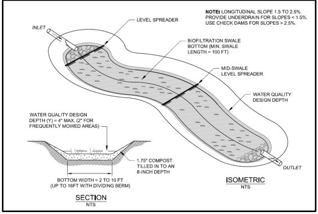
Figure 5.26. Biofiltration Swale Plan and Profile.
