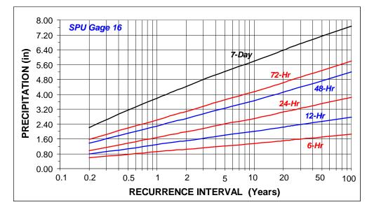
Figure 16. Precipitation-Magnitude-Frequency Estimates for SPU Gauge 16.
