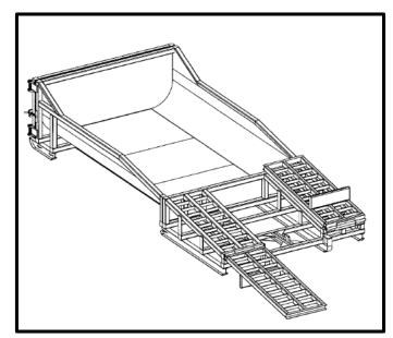
Figure 21. Prefabricated Concrete Washout Container with Ramp.
