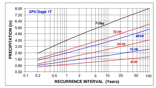
Figure 17. Precipitation-Magnitude-Frequency Estimates for SPU Gauge 17.
