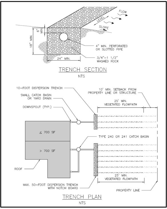
Figure 5.4. Typical Downspout Dispersion Trench.
