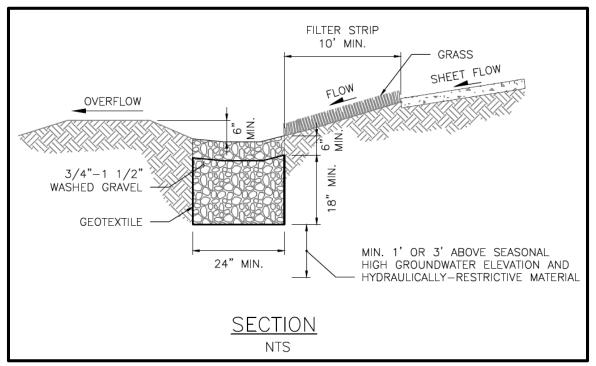
Figure 5.8. Typical Infiltration Trench Receiving Sheet Flow.
