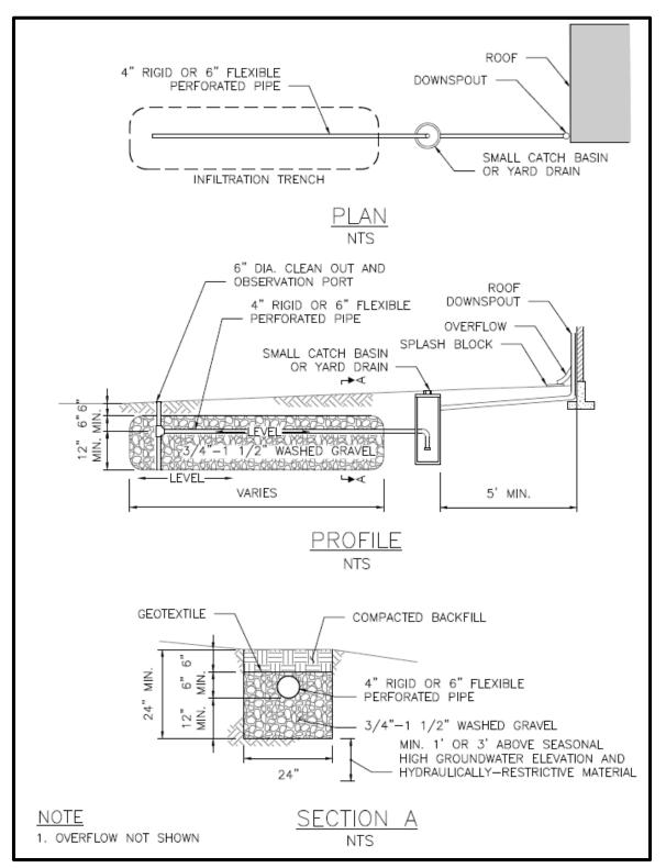
Figure 5.7. Typical Infiltration Trench Receiving Concentrated Flow.
