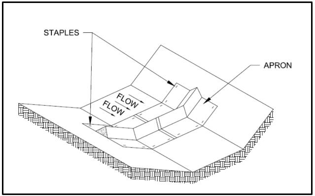
Figure 10. Triangular Silt Dike Cut Section.
