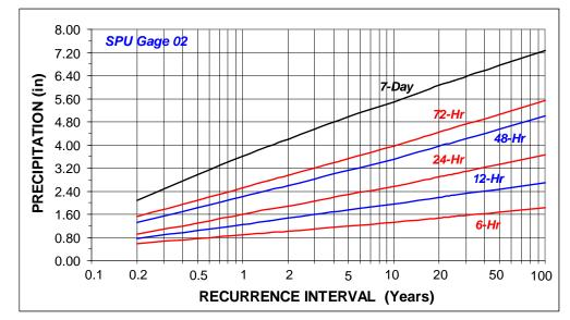
Figure 4. Precipitation-Magnitude-Frequency Estimates for SPU Gauge 02.
