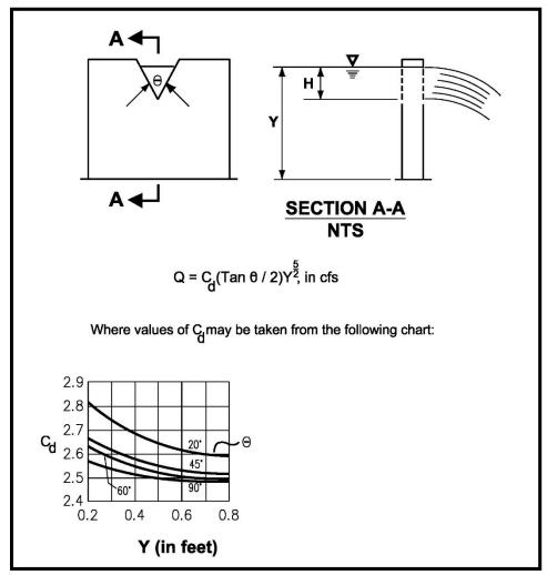
Figure E.2. V-Notch, Sharp-Crested Weir.
