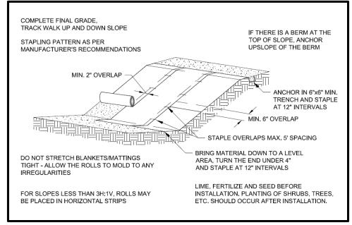
Figure 2a. Mat Installation on Slope.
