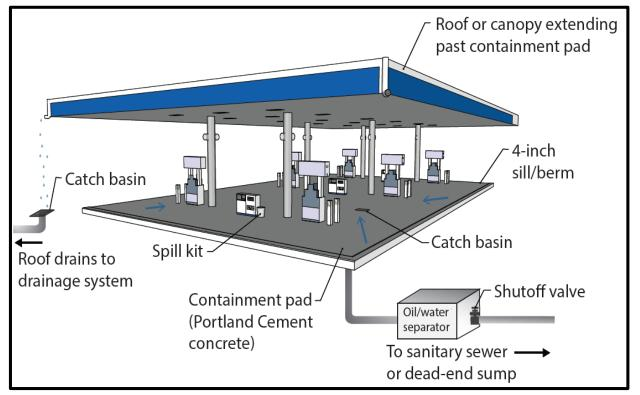
Figure 7. Fueling Island Schematic.
