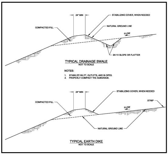
Figure 12. Earth Dike and Drainage Swale.
