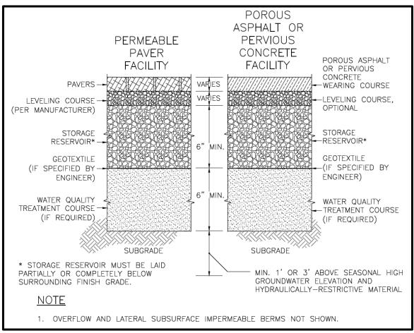
Figure 5.15. Permeable Pavement Facility.
