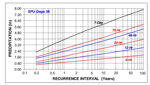
Figure 9. Precipitation-Magnitude-Frequency Estimates for SPU Gauge 08.
