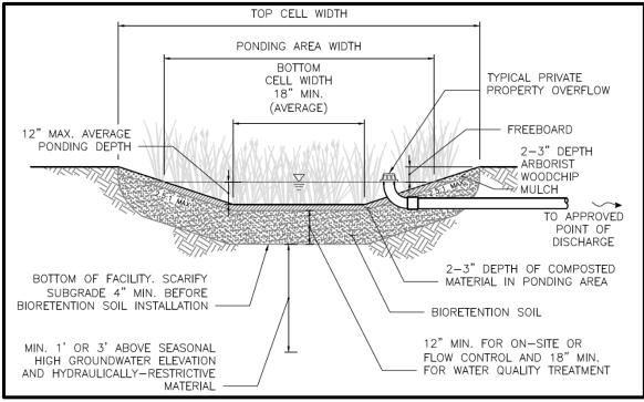
Figure 5.10. Infiltrating Bioretention Facility with Sloped Sides (without Underdrain).
