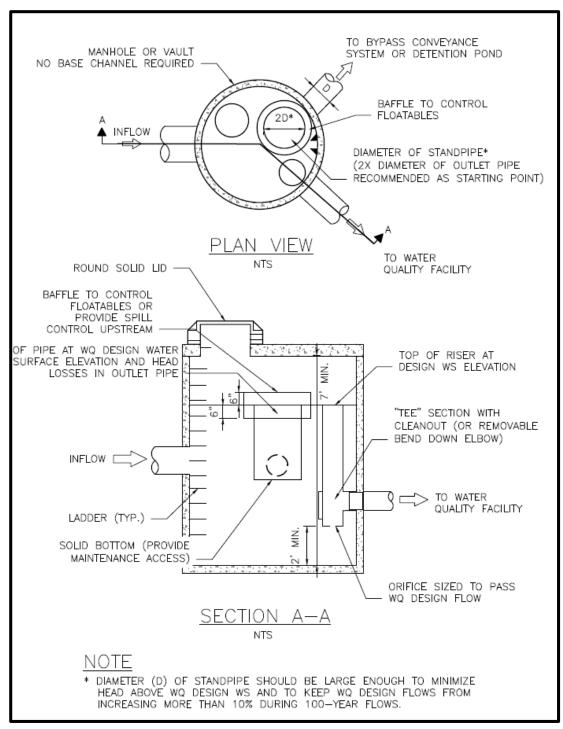
Figure E.5. Flow Splitter Example B.
