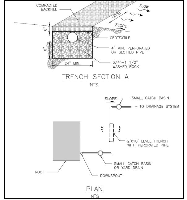
Figure 5.17. Perforated Stub-Out Connection.
