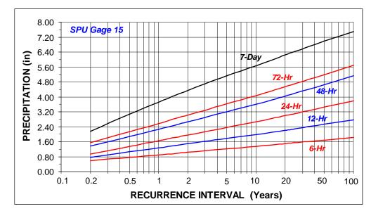
Figure 15. Precipitation-Magnitude-Frequency Estimates for SPU Gauge 15.
