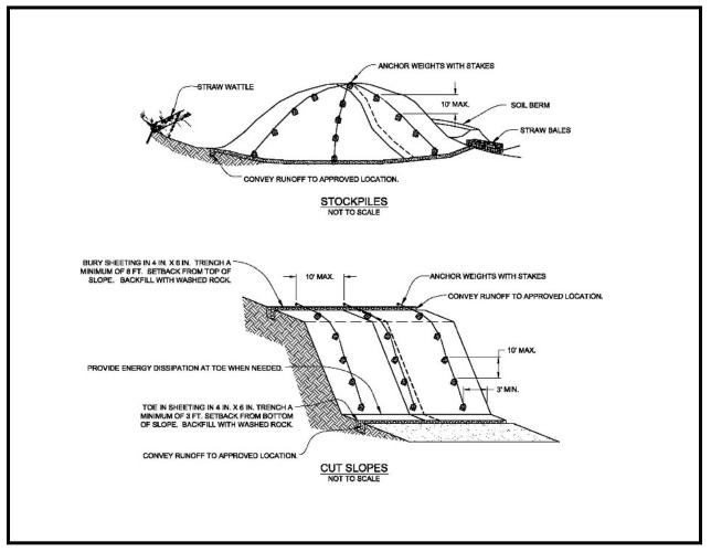
Figure 3. Stockpile Covered with Plastic Sheeting.
