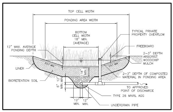
Figure 5.24. Non-infiltrating Bioretention Facility with Sloped Sides.
