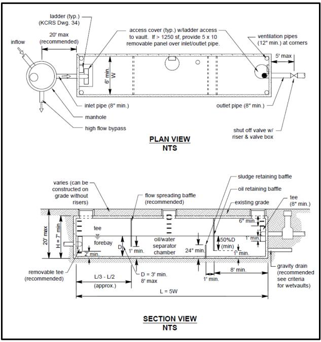
Figure 5.28. Typical API (Baffle Type) Separator.
