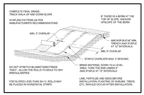
Figure 2a. Mat Installation on Slope.
