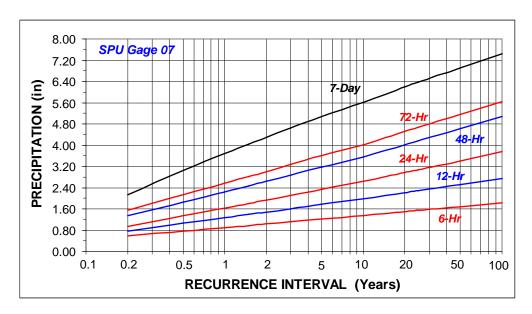
Figure 8. Precipitation-Magnitude-Frequency Estimates for SPU Gauge 07.
