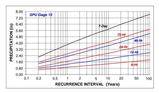
Figure 11. Precipitation-Magnitude-Frequency Estimates for SPU Gauge 10.
