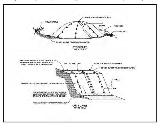
Figure 3. Stockpile Covered with Plastic Sheeting.
