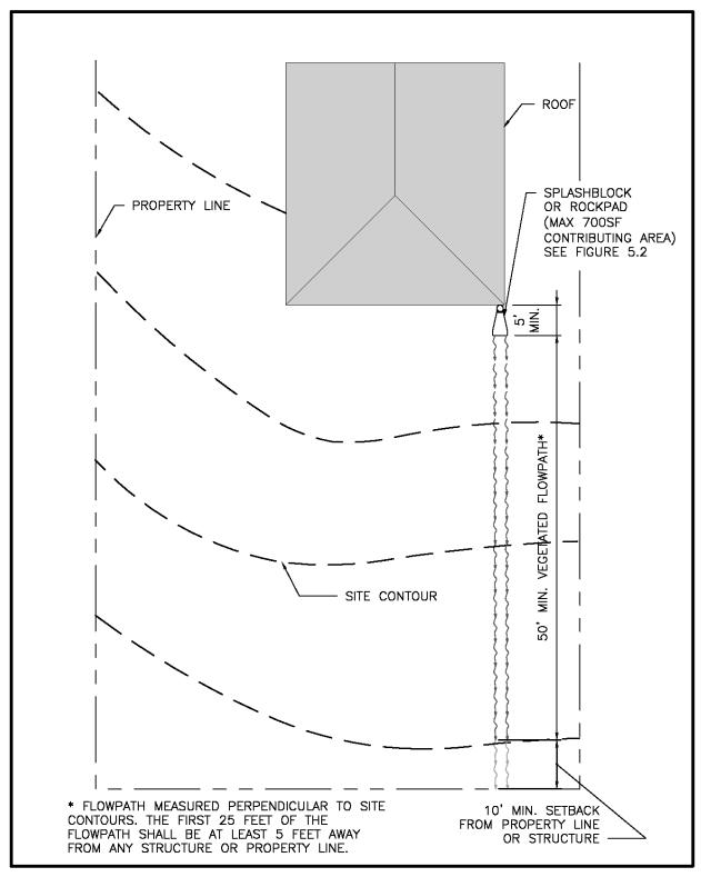
Figure 5.3. Typical Downspout Splashblock.
