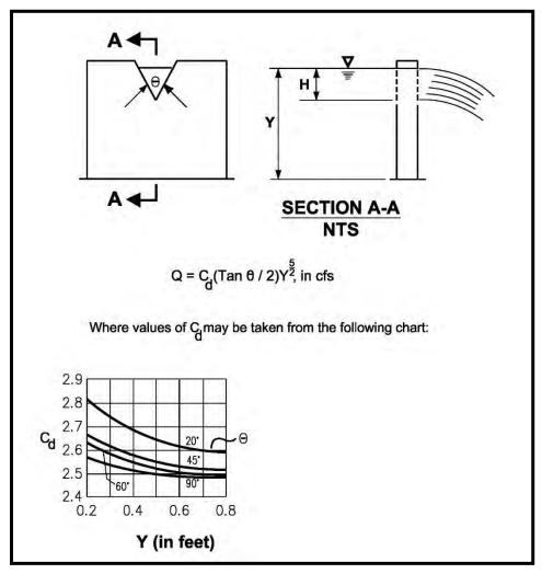
Figure E.2. V-Notch, Sharp-Crested Weir.
