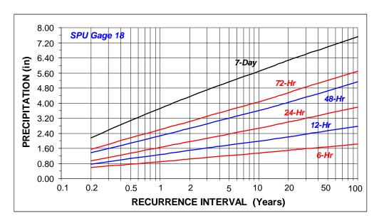
Figure 18. Precipitation-Magnitude-Frequency Estimates for SPU Gauge 18.
