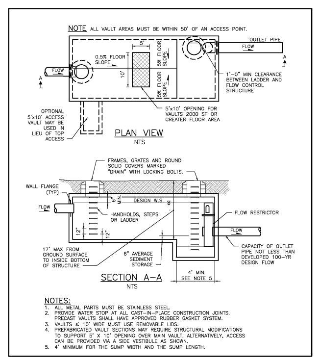
Figure 5.27. Typical Detention Vault.
