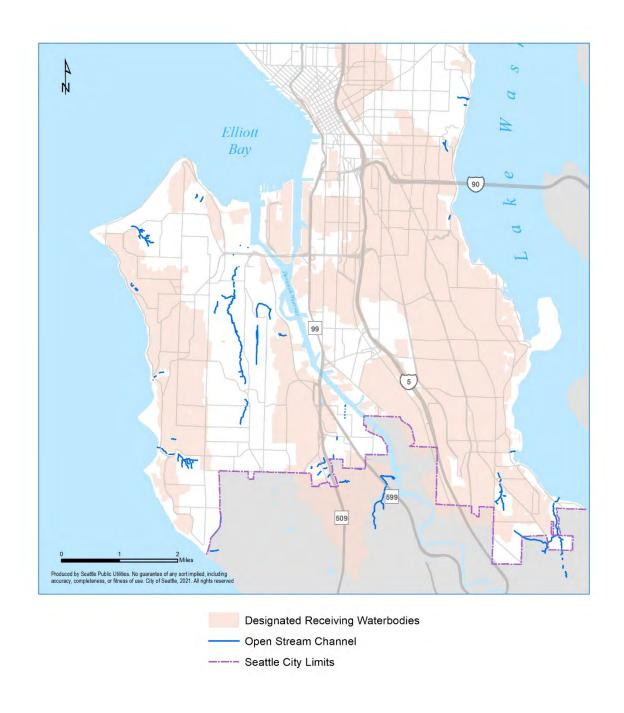
Figure 2.10. South End Designated Receiving Water Drainage Areas.
