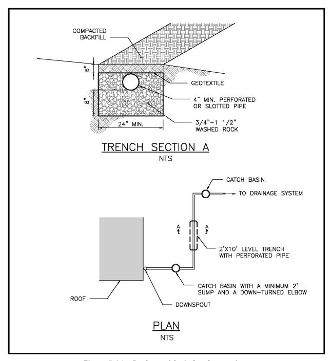
Figure 5.21. Perforated Stub-Out Connection.
