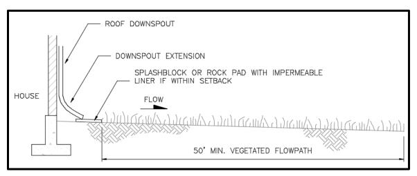
Figure 5.2. Typical Downspout Splashblock Dispersion.
