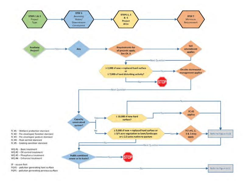
Figure 4.1A. Project Minimum Requirements for Roadway Projects.
