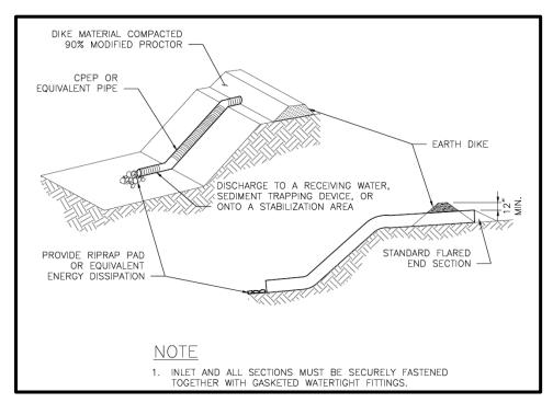
Figure E.8. Pipe Slope Drain Details.
