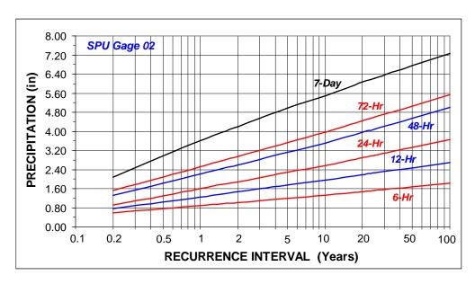
Figure 4. Precipitation-Magnitude-Frequency Estimates for SPU Gauge 02.
