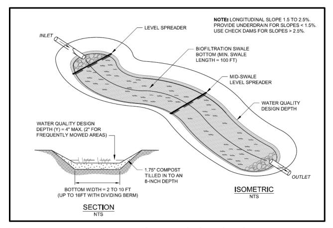
Figure 5.31. Biofiltration Swale Plan and Profile.
