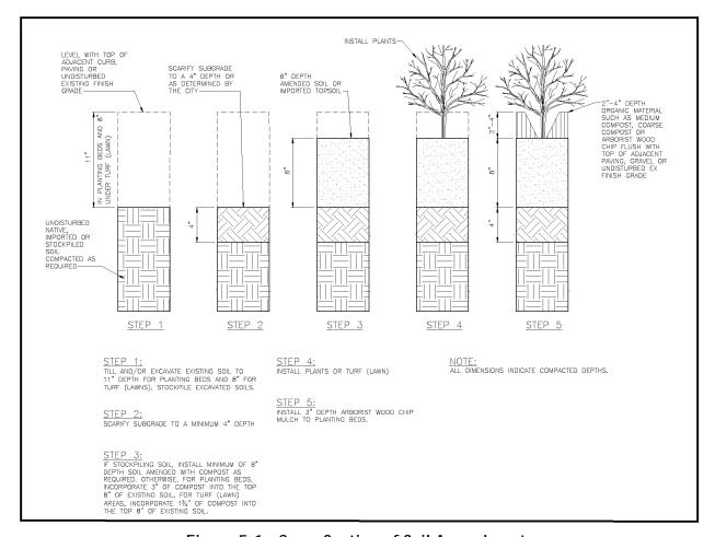
Figure 5.1. Cross-Section of Soil Amendment.
