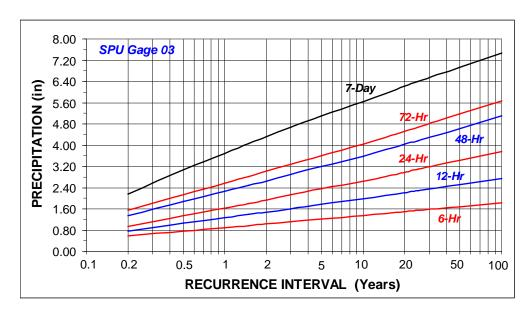
Figure 5. Precipitation-Magnitude-Frequency Estimates for SPU Gauge 03.
