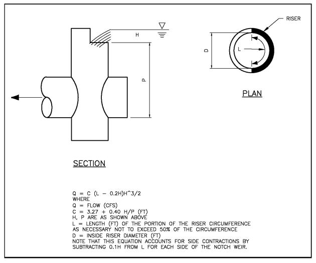
Figure E.3. Rectangular Notch, Sharp-Crested Weir.
