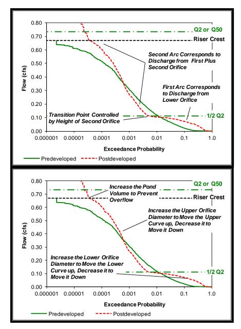
Figure F.7. General Guidance for Adjusting Pond Performance.
