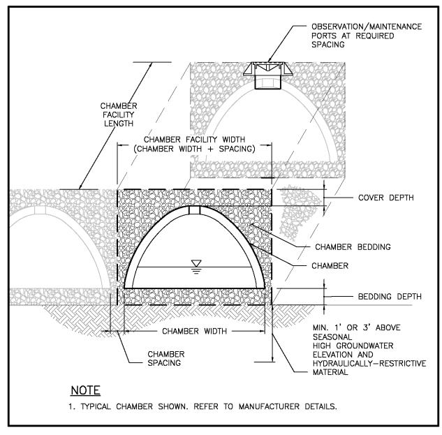
Figure 5.22. Typical Infiltration Chamber/Vault.
