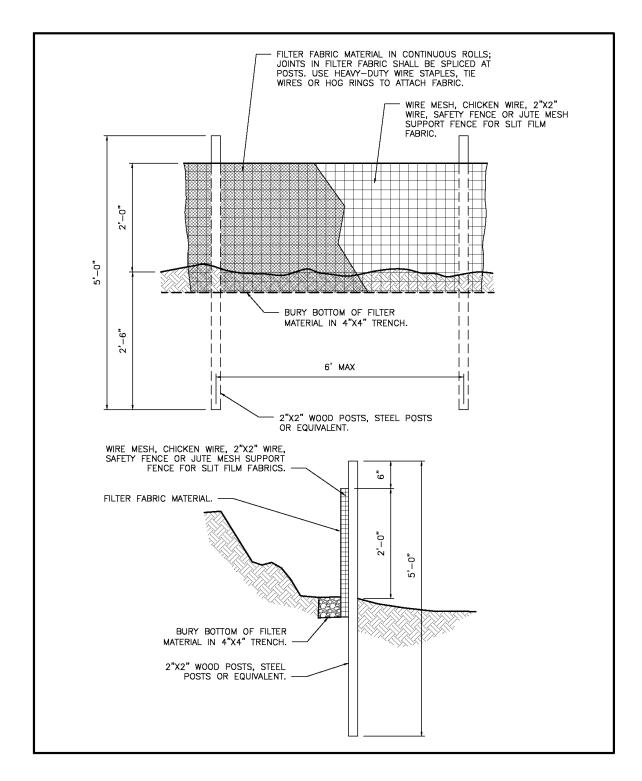
Figure 14. Filter Fence Details.
