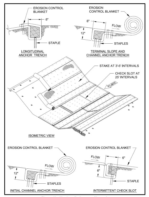
Figure 2b. Mat Installation on a Channel.
