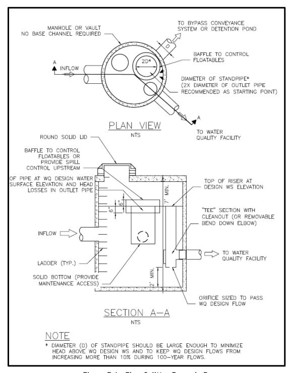
Figure E.6. Flow Splitter Example B.
