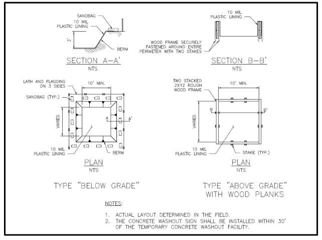
Figure 20. Concrete Washout Facility.
