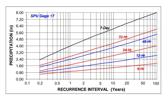
Figure 17. Precipitation-Magnitude-Frequency Estimates for SPU Gauge 17.
