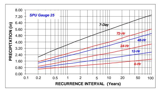
Figure 19. Precipitation-Magnitude-Frequency Estimates for SPU Gauge 25.
