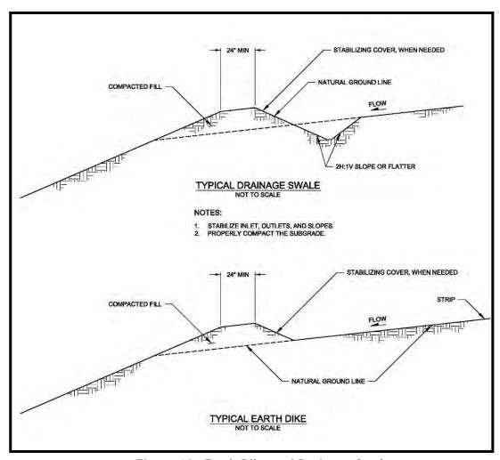
Figure 12. Earth Dike and Drainage Swale.
