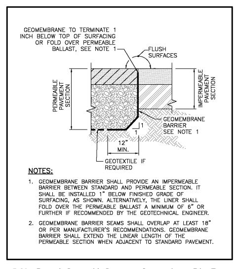
Figure 5.20. Example Permeable Pavement Geomembrane Edge Treatment.
