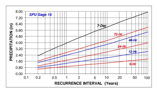
Figure 14. Precipitation-Magnitude-Frequency Estimates for SPU Gauge 14.
