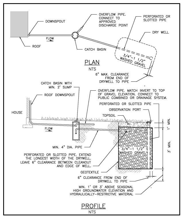
Figure 5.10. Typical Infiltration Drywell.
