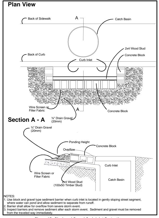
Figure 15. Block and Gravel Curb Inlet Protection.
