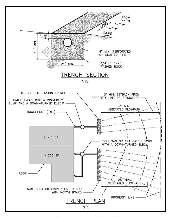
Figure 5.4. Typical Downspout Dispersion Trench.
