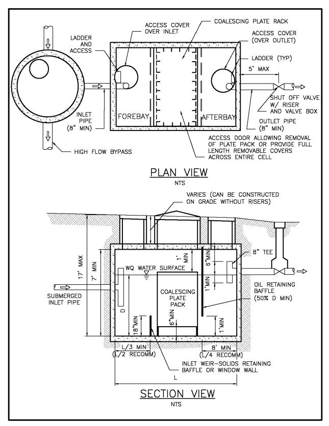
Figure 5.34. Typical Coalescing Plate Separator.
