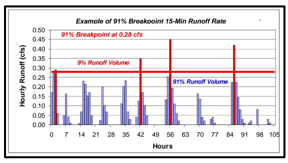
Figure F.11. On-Line Water Quality Treatment Discharge Example.
