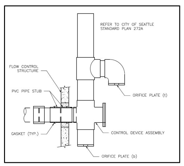
Figure E.1. Simple Orifice.
