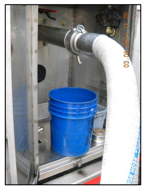
Figure 8. Temporary Containment Device Placed Under a Hose Connection.
