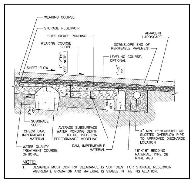
Figure 5.18. Example Permeable Pavement Facility with Checkdams.
