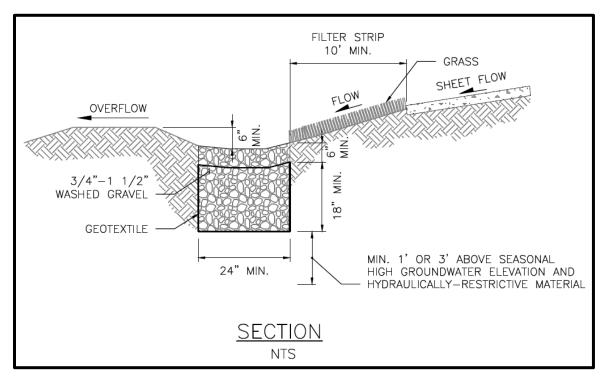
Figure 5.9. Typical Infiltration Trench Receiving Sheet Flow.
