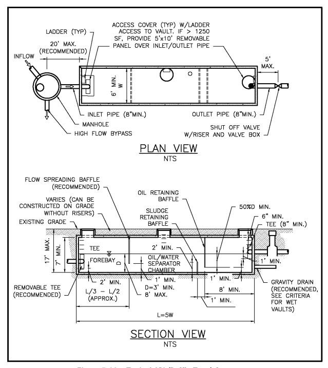
Figure 5.33. Typical API (Baffle Type) Separator.
