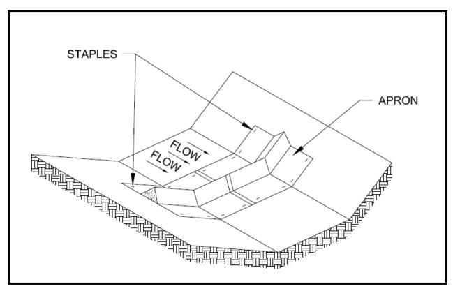
Figure 10. Triangular Silt Dike Cut Section.
