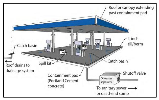
Figure 3. Fueling Island Schematic.
