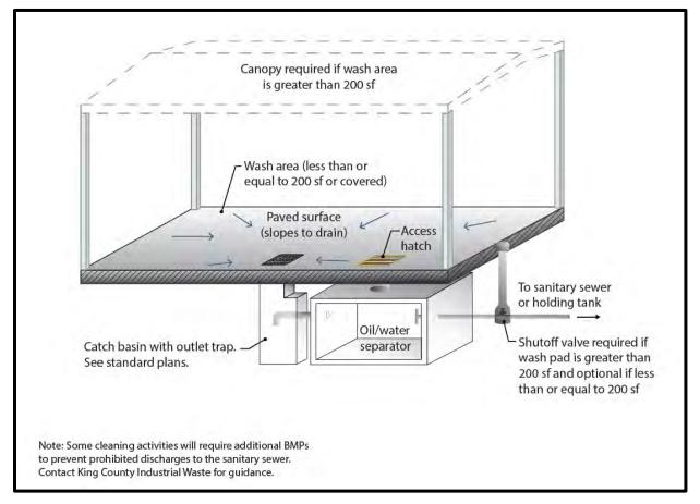
Figure 7. Schematic of Wash Pad with Sump.
