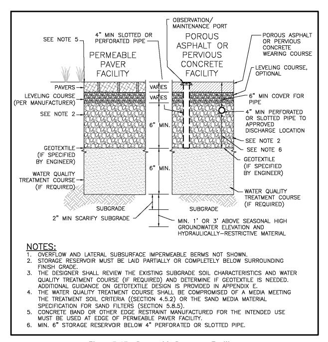
Figure 5.17. Permeable Pavement Facility.
