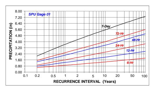
Figure 3. Precipitation-Magnitude-Frequency Estimates for of SPU Gauge 01.
