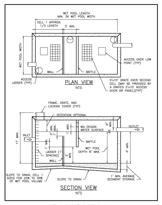
Figure 5.32. Typical Wet Vault.
