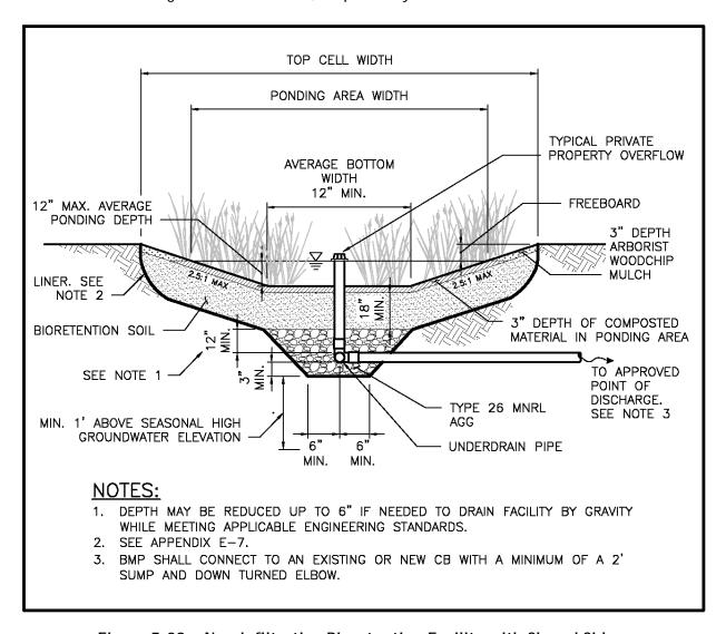
Figure 5.29. Non-infiltrating Bioretention Facility with Sloped Sides.
