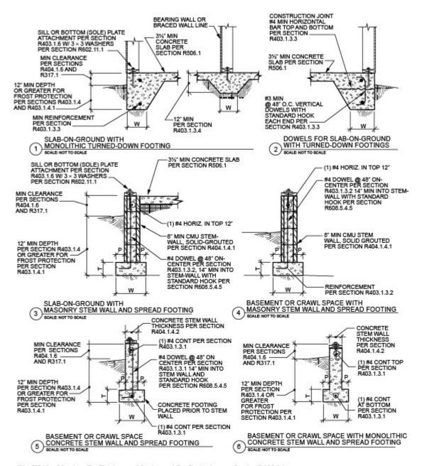
W = Width of footing, T = Thickness of footing and P = Projection per Section R403.1.1 NOTES:
