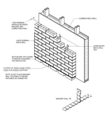
FIGURE 308.2(2) WALL PROTECTOR CLEARANCE REDUCTION SYSTEM
