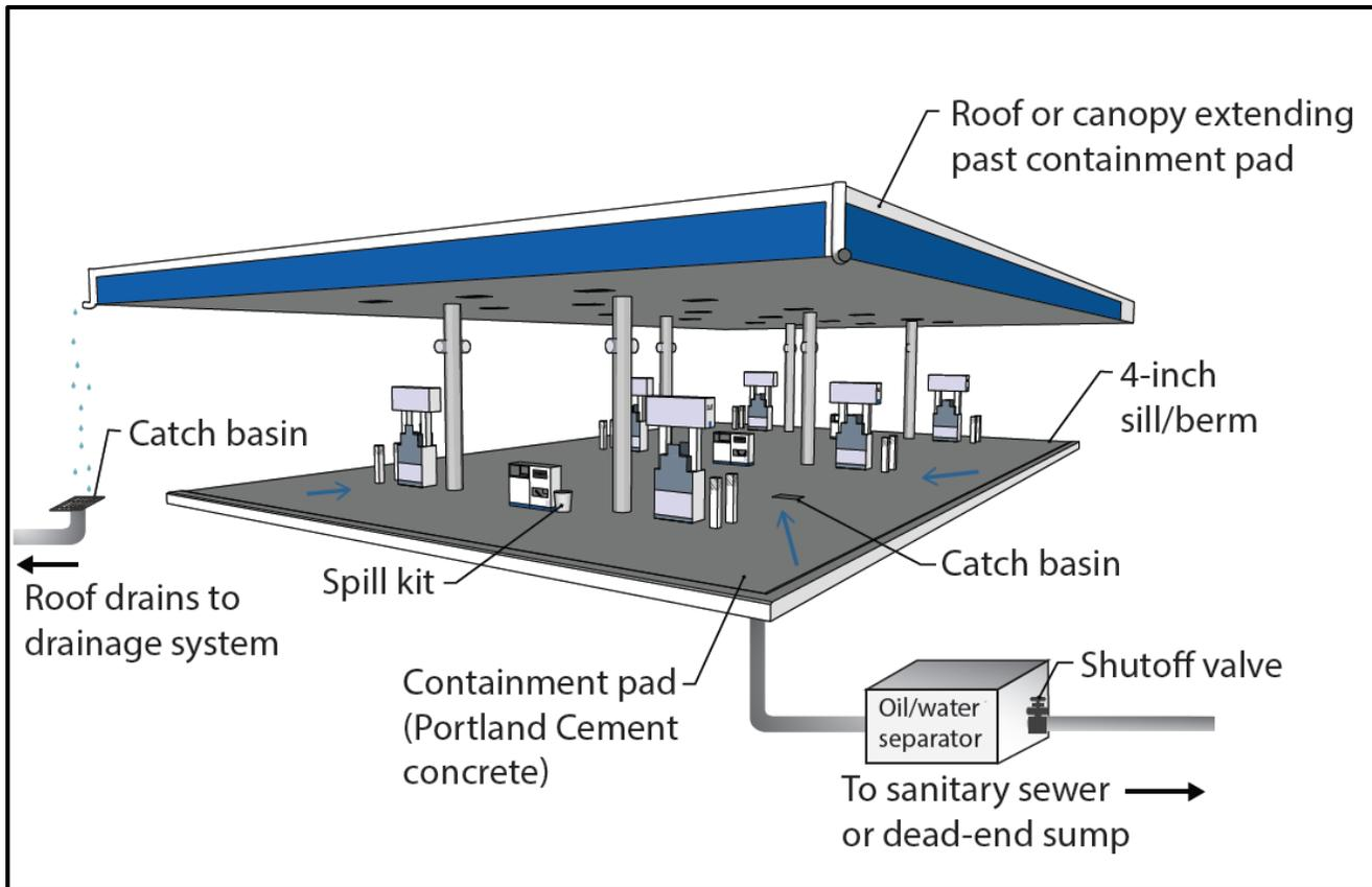
**Figure 7. Fueling Island Schematic.**
