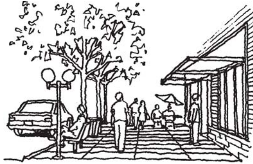
A sidewalk providing clear sidewalk space, street furniture, and an acceptable distance between streetscape amenities and vehicle travel lanes.
