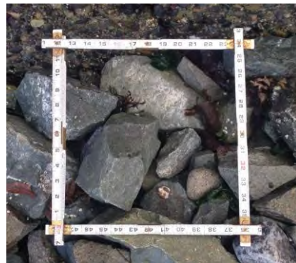
G. Quarry spalls at north park boundary
