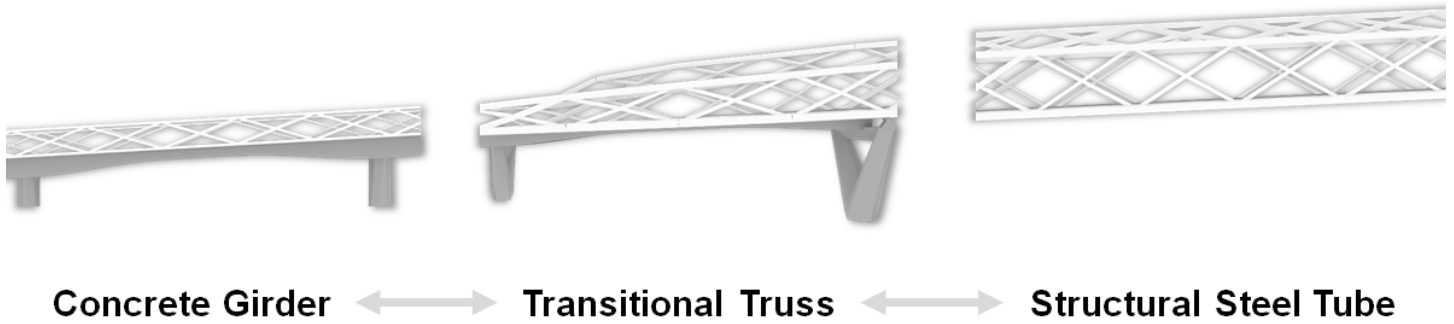
Figure 5. Proposed bridge structure
