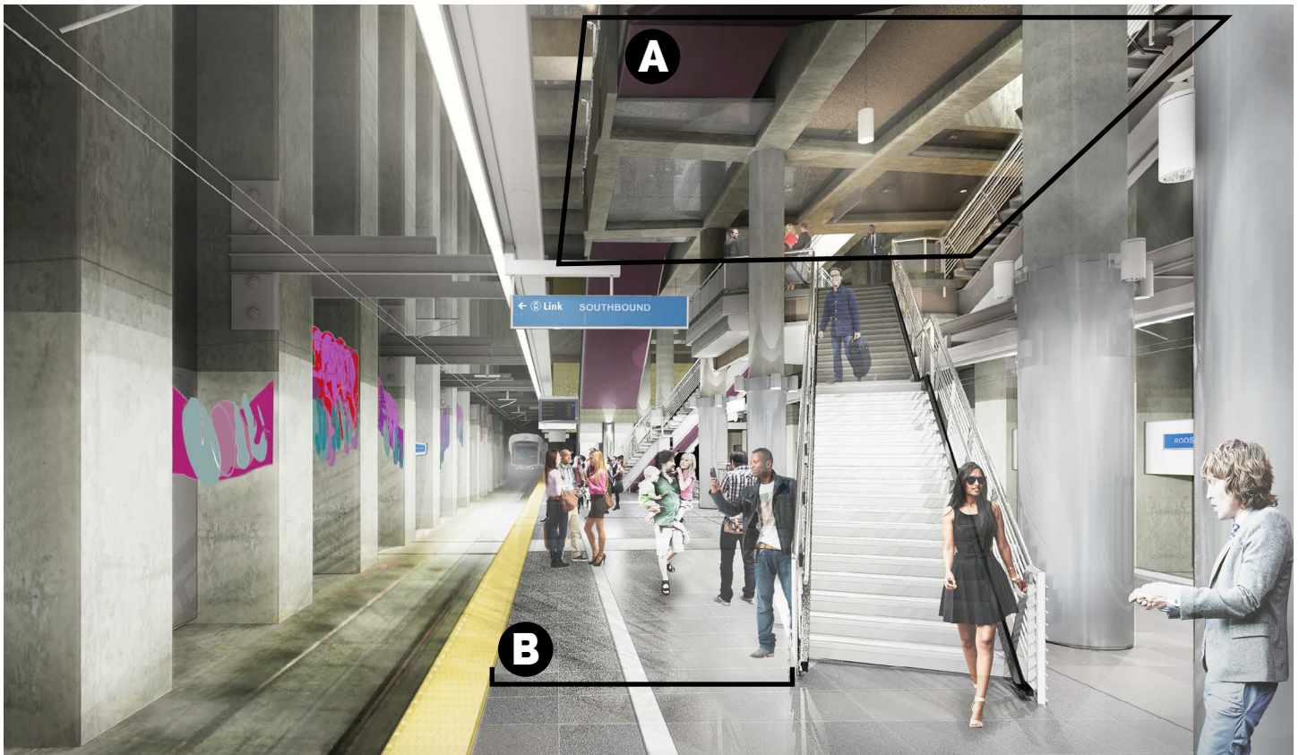
Figure 3. This perspective highlights two LRRP comments. First, they saw a conflict between geometry of the mezzanine and the expression of the columns and beams that support the station box (A). Second, they asked that Sound Transit provide studies demonstrating the distance between the stair landing and platform edge was adequate (B).
