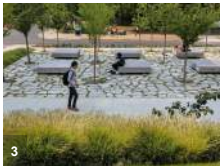
3 • Use different types of paving to imply different uses of space
