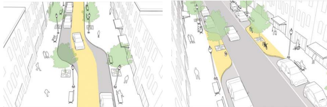
Traffic-calming chicane design from SDOT Streets illustrated.
