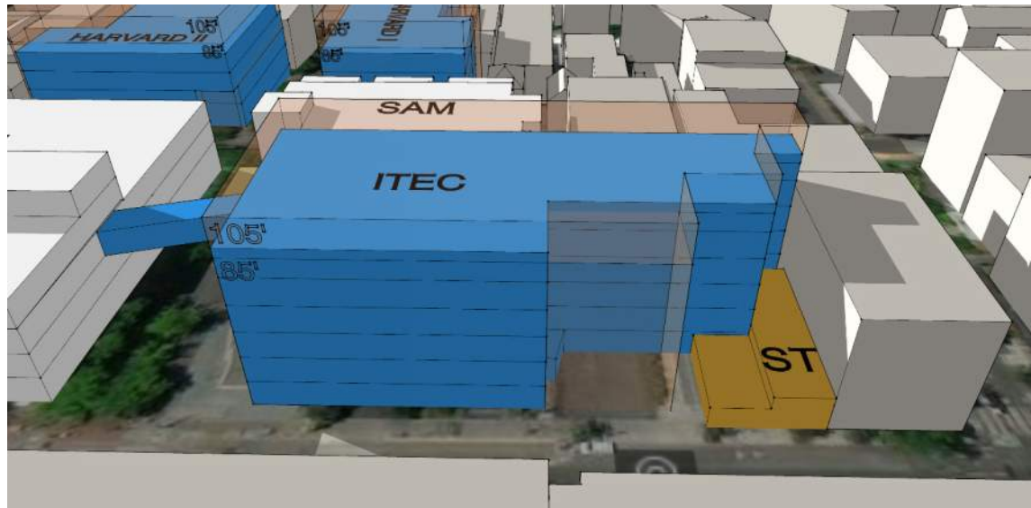
ITEC – Six stories and approximately 95 feet
