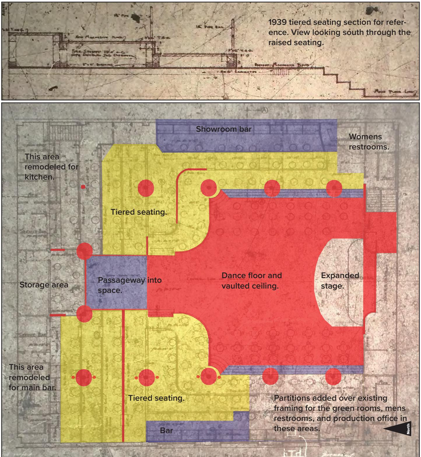
**Figure 6.** Second floor analysis plan. The 1939 remodel plan is the base drawing with overlaid color coding to show what remains today from the original design. The core volume, dance floor, raised seating, columns, proscenium, and fly loft all remain. Refer to the character defining features and spaces section in the description for a full list of the features.
