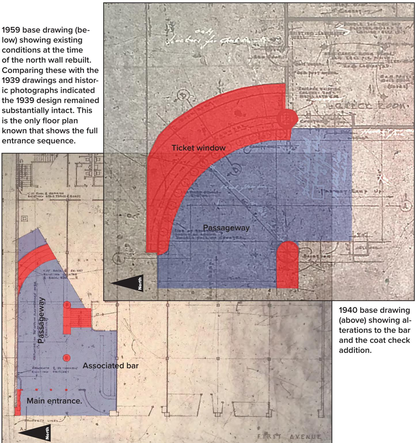
1940 base drawing (above) showing alterations to the bar and the coat check addition.
