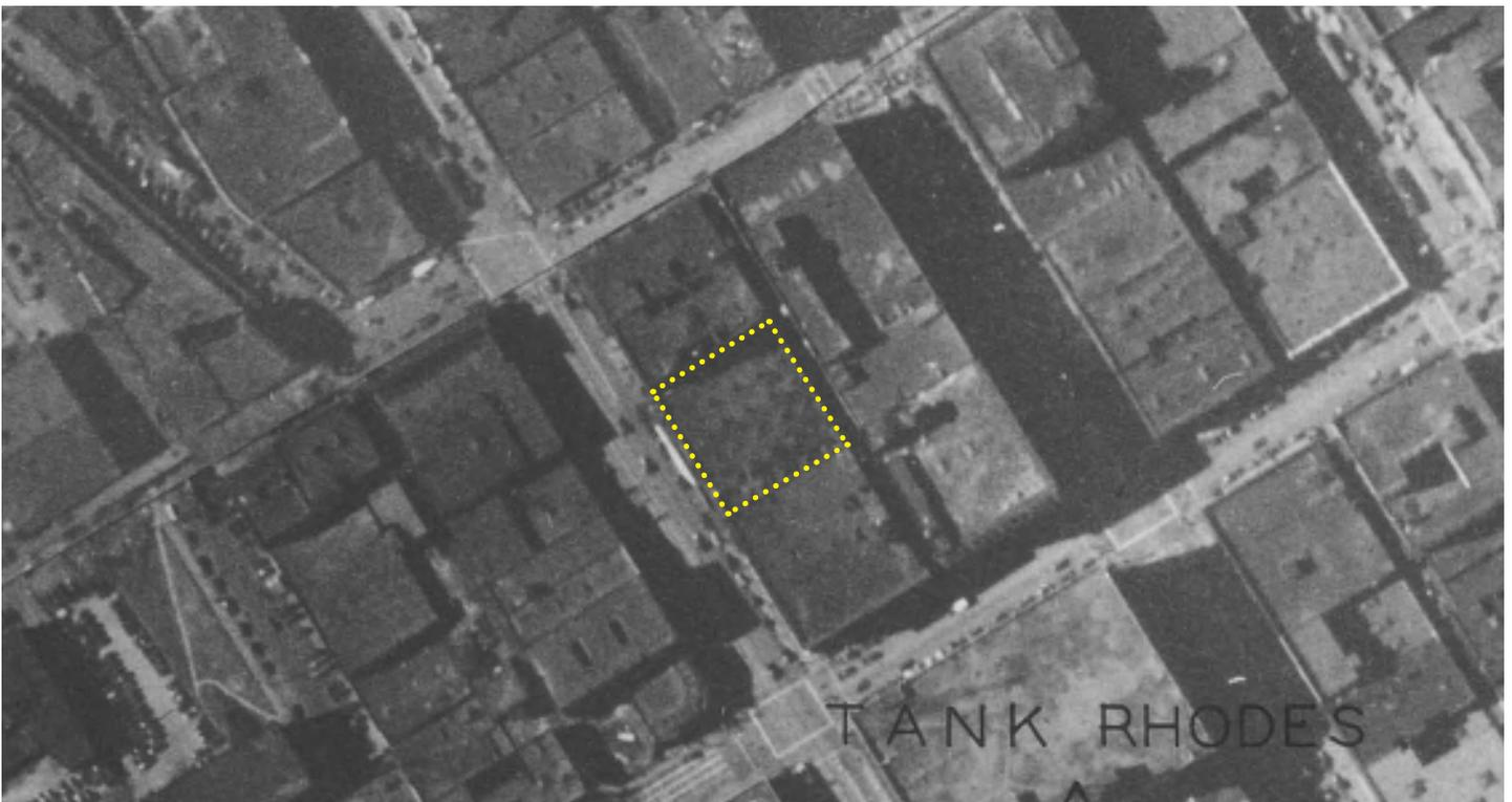
**Figure 74.** 1937 King County aerial showing the building (outlined in yellow dots) prior to the 1939 remodel. Note the elevated central truss roof portion for the vaulted ceiling at the second floor was part of the 1939 remodel.
