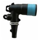
established or broken by engaging or separating the connector at the operating interface. Suitable for use on 26.4 kV, 4-wire, solidly-grounded systems and 5 kV systems. Because of high fault duty, connectors rated 200 A continuous are not appropriate for network systems. Network systems should be constructed with connectors rated 600 A (or 900 A) continuous.
