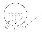
this bushing typically covered with heat shrink to prevent accidental connection
