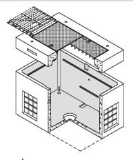
**Dimensions** Outside Inside Stock No. Description Length Width Height Length Width Height 014370 Base 7' 0" 4' 8" 4' 0" 6' 6" 4" 2" 3'8" 7' 0" 014371 Cover, with solid hatch 4' 8" 1'0" 6'6" 4" 2" 014372 Assembly, base and cover 7' 0" 4' 8" 5'0" 6'6" 4" 2" 4' 8"
