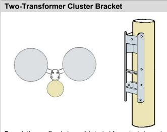
Description: Brackets are fabricated from steel channel
