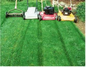
Push mowers (left) and conventional power mowers (right) leave clippings scattered on the surface, where they break down in a week or so. Modern electric and gas mulching mowers (center) blow mulched clippings down to the ground, making free fertilizer and leaving a clean-looking lawn.
