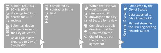
All Record Drawings are created from As-Built Drawings, uploaded to GIS and archived into the Engineering Records Center and Virtual Vault by City of Seattle staff.
