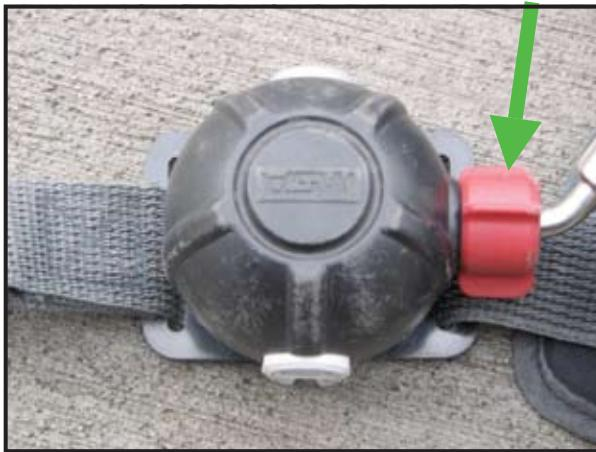
The Emergency Bypass (green arrow in pic) is located on the right side of the second stage regulator as if the user were wearing it. The Emergency Bypass is designed to be used should there be a malfunction of the second stage regulator (inability to breathe due to malfunction).
