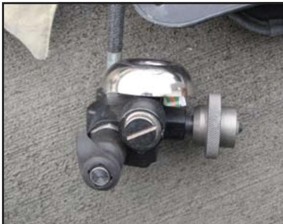
**The Audi-larm rings when there is about 25% of the cylinder's rated service time remaining.** The alarm will also ring when the cylinder valve is first opened. This provides the user the audible alarm indication that the system is charged and alarm is cocked. A high pressure hose delivers high-pressure from the alarm to the first stage regulator.
