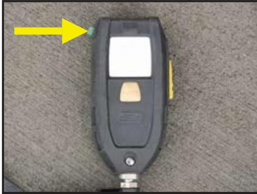
The top green **MODE** button (yellow arrow in pic) is used for unit system information. Pressing it 1 time will light up the LCD screen and refresh or relight the HUD receiver on the face-piece. While the screen is still lit, pressing the MODE button again will change the LCD screen from remaining cylinder pressure to calculated remaining service life of the cylinder. This service life number can change based on breathing/usage
