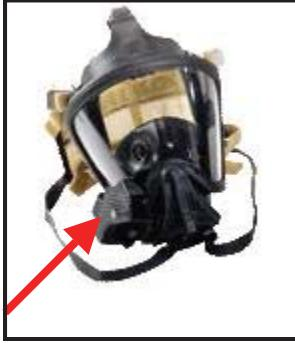
The Night-Fighter Heads Up Display (HUD) receiver (red arrow in pic) on the face-piece shows the air cylinder content in one quarter increments, from a full cylinder to an empty cylinder by means of LED light pattern. These lights are seen through the lower right corner of the face-piece lens as the user would wear it.
