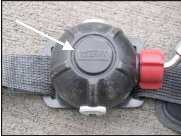
This is a pressure demand regulator, which keeps a positive pressure in the face-piece at all times. Removal of the second stage regulator by depressing the upper and lower release buttons will stop the airflow. To restart the regulator, re-insert the second stage regulator into face-piece and inhale sharply. The button automatically disengages the diaphragm, allowing air to flow to the face-piece. The
