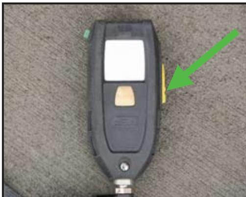
The **RESET/OFF** button (green arrow in pic.) located on the side of the unit resets the device from the full ALARM mode (2 presses). It also shuts off the unit after the cylinder valve is closed and all air pressure is bled from the unit (2 presses).
