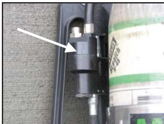
The first stage regulator keeps the pressure to the mask-mounted regulator at approximately 80 psi throughout the entire operating pressure range of the cylinder. This regulator has a redundancy feature to minimize the possibility of a first stage failure. This regulator will vent any excess pressure sent to the regulator from the cylinder.
