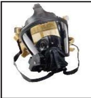
Your personal face-piece is a small, medium or large size. The lens is super-hardcoated polycarbonate and the lens has a melt temperature of 500 degrees F° to meet NFPA 1981 standard. Applications have shown these to soften and lose structural integrity when prolonged exposures around 300+ degrees F°. are encountered. An inhalation check valve keeps ambient moisture outside of the mask mounted regulator. The exhalation valve is a pressure demand type designed
