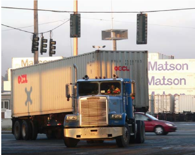
Container trucks require a larger turning radius than many other vehicles.
