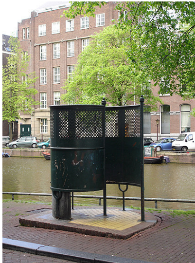
One example of a snail entry restroom in Europe. Snail-type entries can be used on more substantial structures, for both the main entry and for individual stalls.
