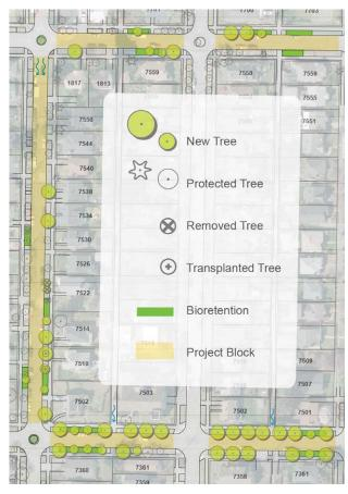
Figure 10. Bioretention and Street Tree Siting
