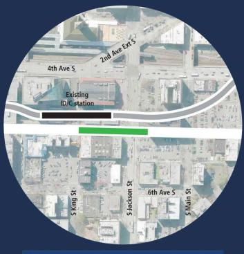
Station location alternative (straddle S Jackson St) Note: applicable to both cut and cover and bored tunnel alternatives
