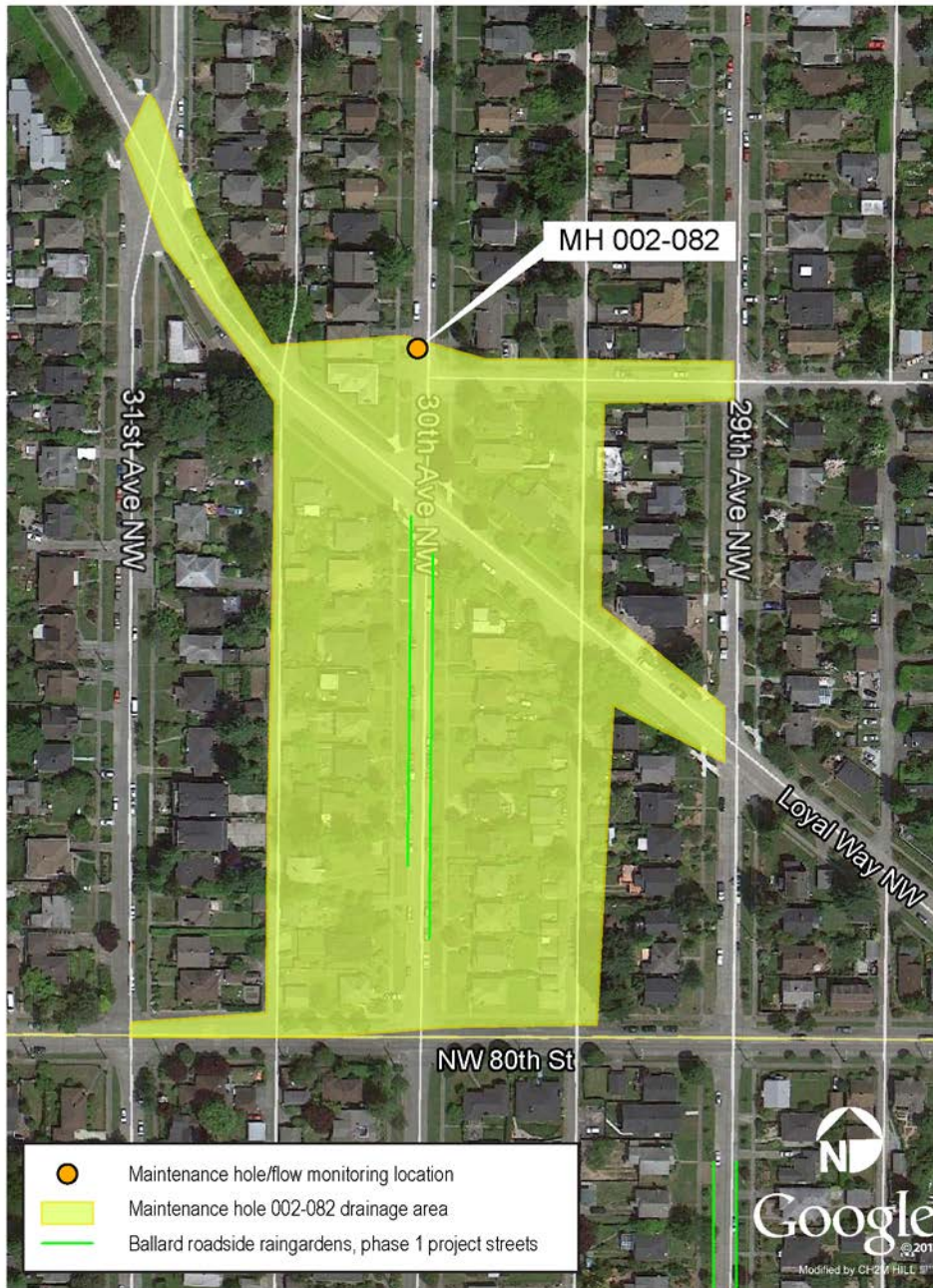
Figure 12. 30th Avenue Drainage Area to Flow Monitor in MH 002-082
