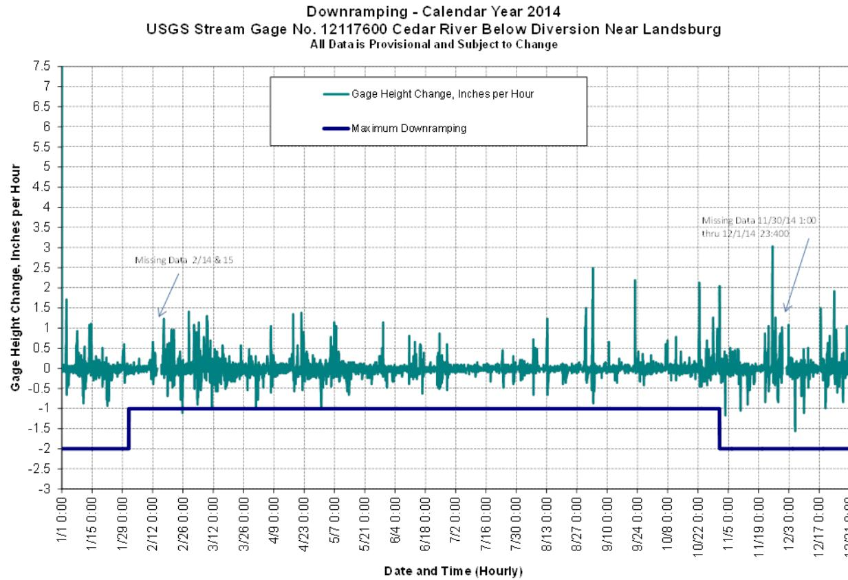
**Figure 8.4 – Downramping Flows below Powerhouse Compliance Graph**
