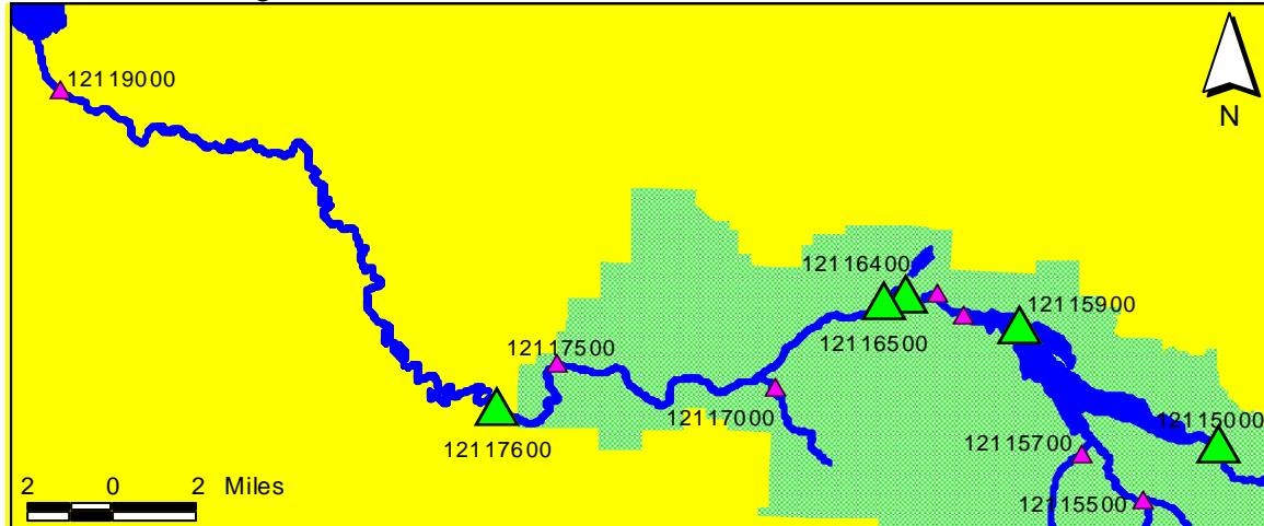
**USGS Gaging Station 12117600** – Cedar River below Diversion near Landsburg, Washington. Located at River Mile 20.4, this gage measures regulated stream flow downstream of Landsburg Diversion Dam. This is the measuring point for flows and downramping rates immediately below the Landsburg Diversion Dam, as required in Section B and sub-section C.2.c in the IFA.
