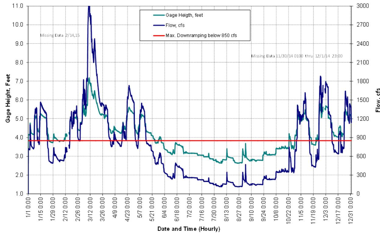
**Figure 8.3 – Downramping Rate of Change Below Landsburg Compliance Graph**
