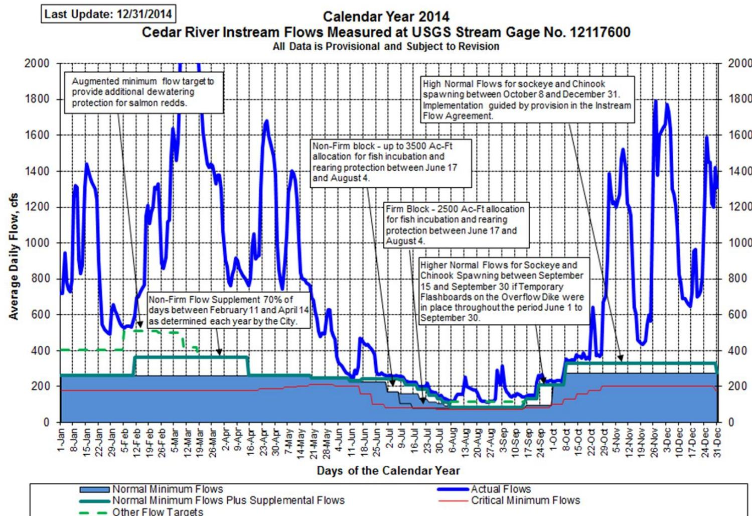
**Figure 8.2 – Downramping Flows Below Landsburg Compliance Graph**
