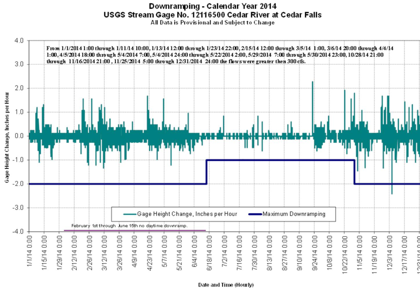
**Figure 8.6 – Downramping Flows below Masonry Dam Compliance Graph**
