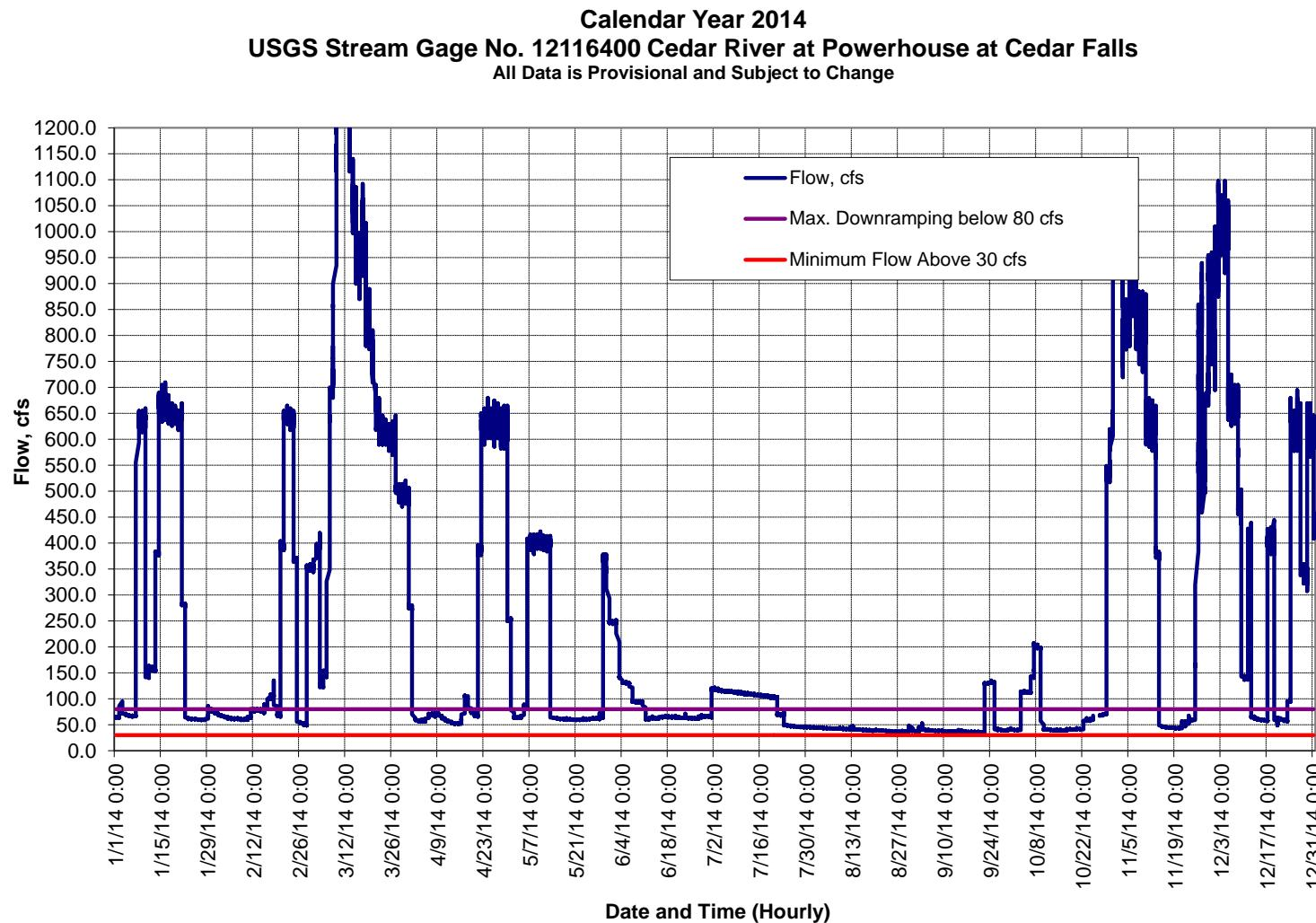
**Figure 8.7 – Downramping Rate of Change Below Masonry Dam Compliance Graph**
