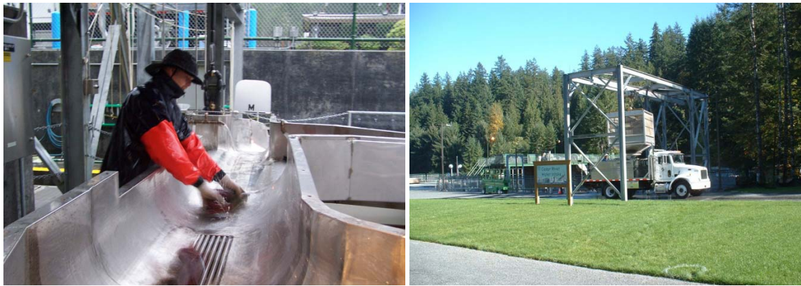
Figure 2: Sorting table operation and fish hopper on top of fish transport truck.
