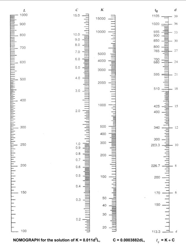
7-17.3(4)F HYDROSTATIC TEST FOR SANITARY SEWER FORCE MAINS
