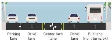
The Phase 2 street layout will typically include a parking lane (either on the west or east side of the street), travel lane in each direction, center turn lane, and bus lane.
