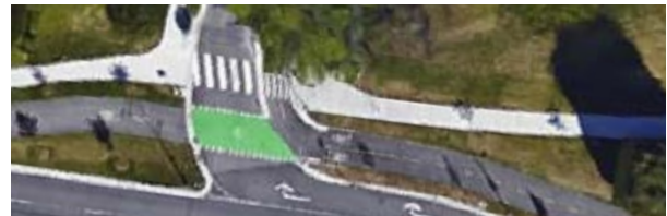
Separated bicycle and pedestrian facilities with marked pedestrian crossings of the bicycle trail
