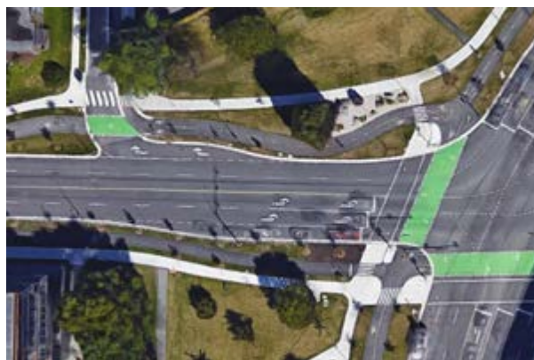
Separated pedestrian/bicycle paths through intersections (Burrard St in Vancouver, BC)
