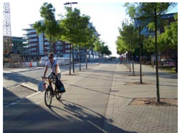
Bicycles and pedestrian spaces distinguished with paving
