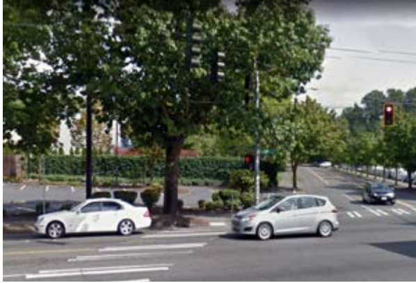
The existing APS on the north side of S Bayview St encourages people to use this crossing, but the alignment with the tree makes it very unsafe for people who are blind or deafblind.
