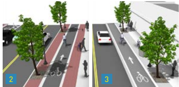
Examples of PBLs: 1) At street level and buffered with paint and bollards, 2) Raised above street level and buffered from vehicles and pedestrians, and 3) Raised above street level and separated from pedestrians.
