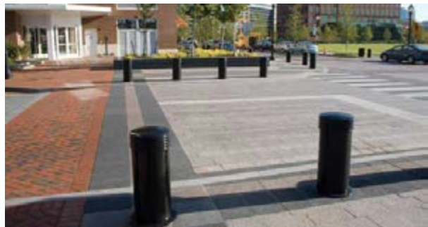
Tactile ground treatments can clarify bicycle and pedestrian space.
