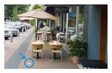
Example of pavement markers. SDOT-provided markers will be 6 inches in diameter and must be located every 10 feet along the entire perimeter of the café.
