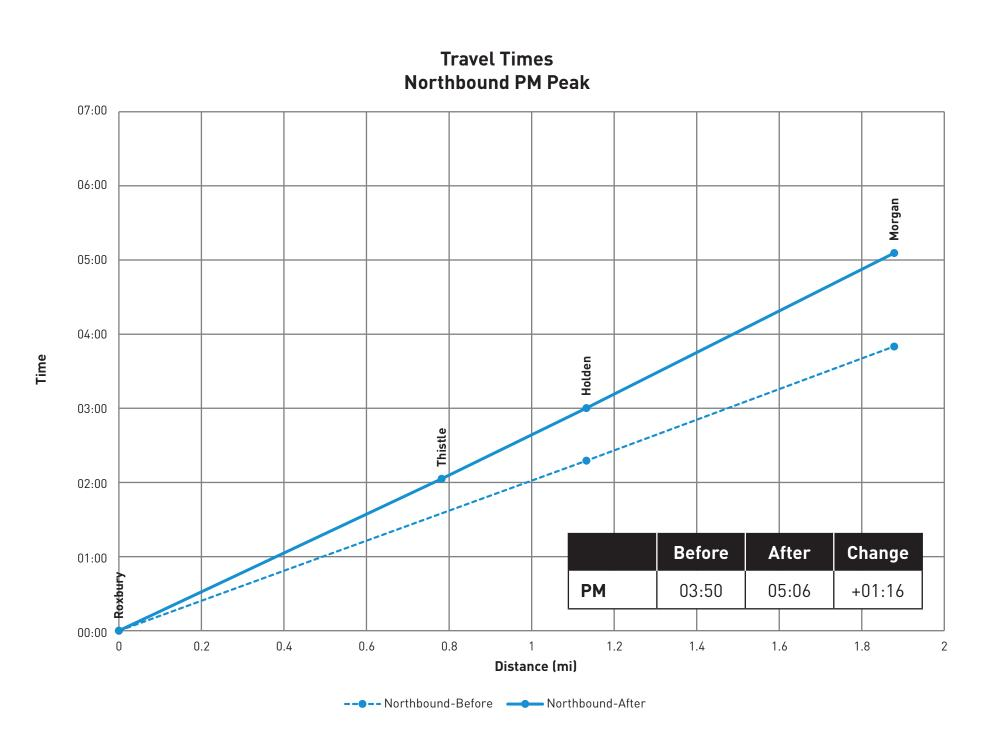
Longer queues can develop when the Seattle Fire Department deploys to emergencies from Station 39 at SW Holden Street. However, our signals are designed to clear these queues in one to two signal cycles.
