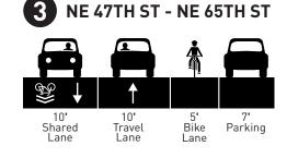
Cross sections are looking north. Illustrations are conceptual. Actual widths at intersections will vary.
