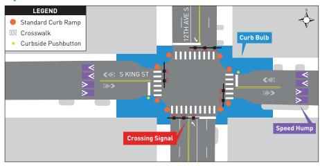
Use curbside pushbutton to cross when biking, removes about 4 parking spaces
