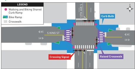
Add two raised crosswalks, use curb bulb when biking to cross with pedestrians, removes about 6 parking spaces
