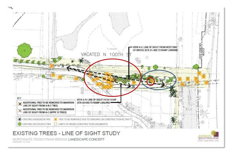
There was no line of sight between sight line C and A. The tree canopy is thick and blocks the area where the end of bend in the bridge will be. This would reduce safety for pedestrians and create areas of concealment for abnormal users. The trees blocking this sight line should be removed to increase natural surveillance.
