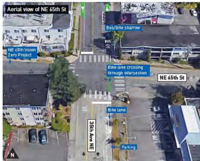
Conceptual view of intersection at NE 65th St; image not to scale
