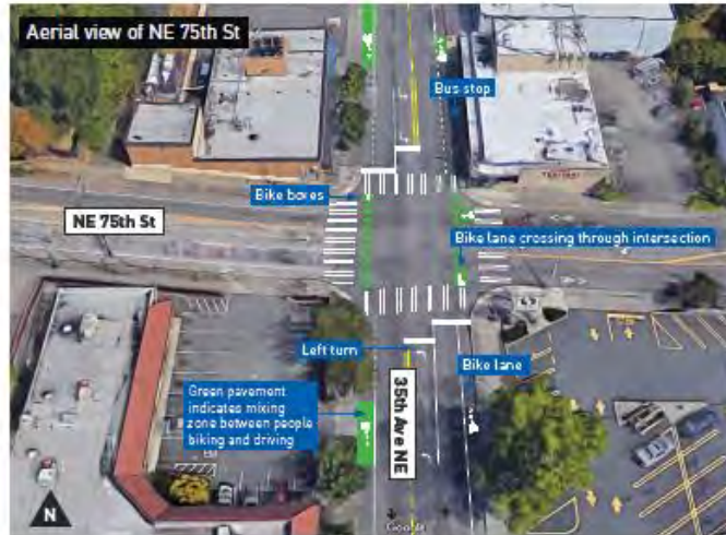
Conceptual view of intersection at NE 75th St; image not to scale
