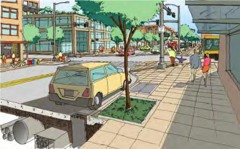
Conceptual sketch of the public right-of-way in a neighborhood business district showing underground utilities.
