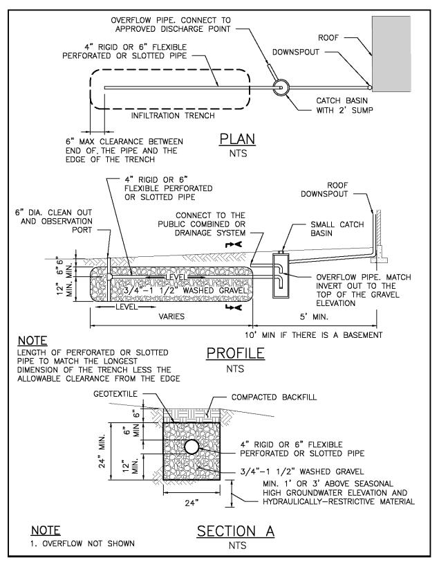
Figure 5.8. Typical Infiltration Trench Receiving Concentrated Flow.
