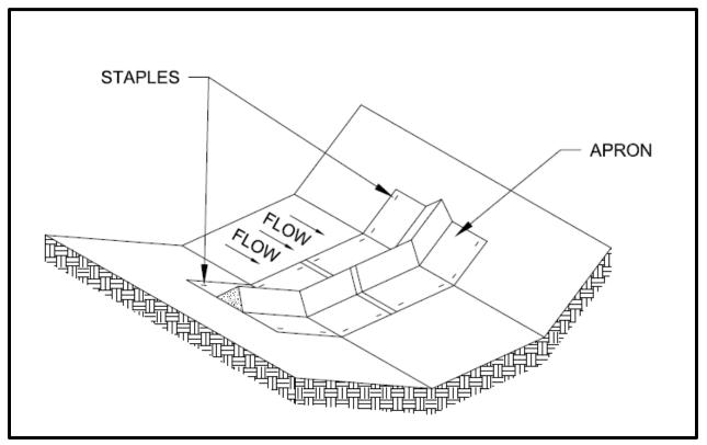
Figure 10. Triangular Silt Dike Cut Section.
