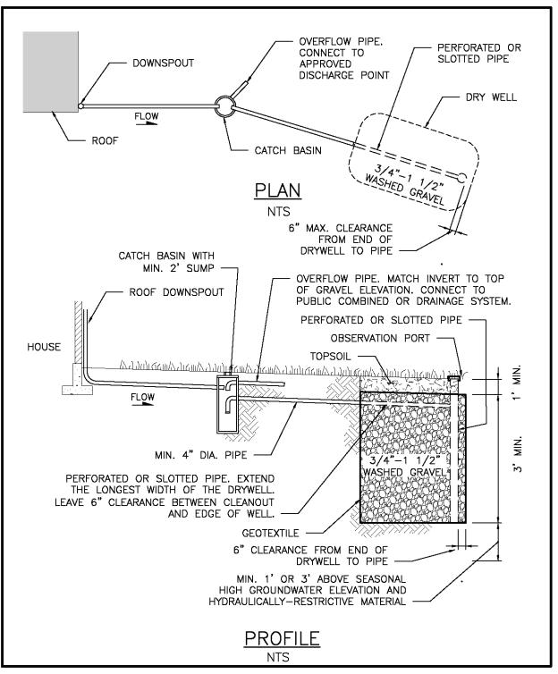
Figure 5.10. Typical Infiltration Drywell.
