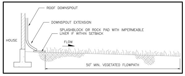
Figure 5.2. Typical Downspout Splashblock Dispersion.
