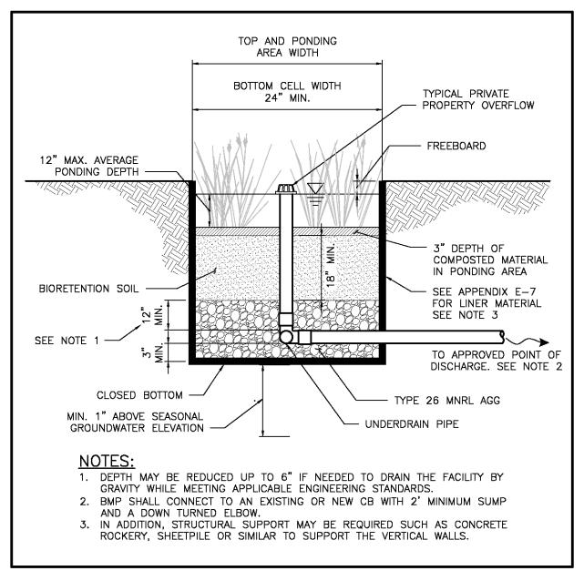
Figure 5.30. Non-infiltrating Bioretention Facility with Vertical Sides.
