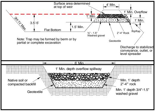
Figure 19. Cross Section of Sediment Trap and Outlet.
