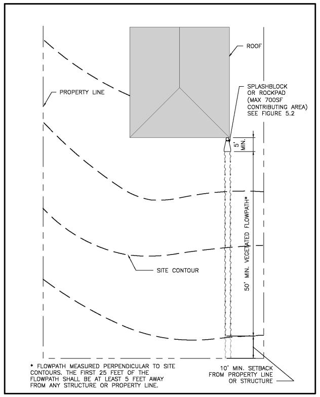
Figure 5.3. Typical Downspout Splashblock.
