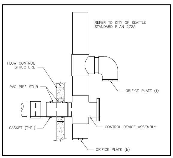
Figure E.1. Simple Orifice.
