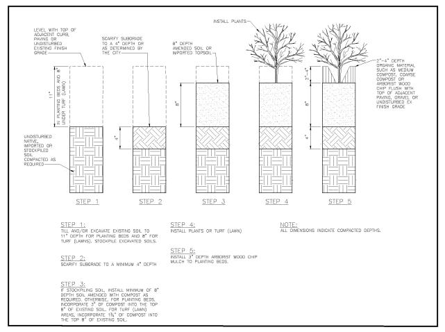
Figure 5.1. Cross-Section of Soil Amendment.
