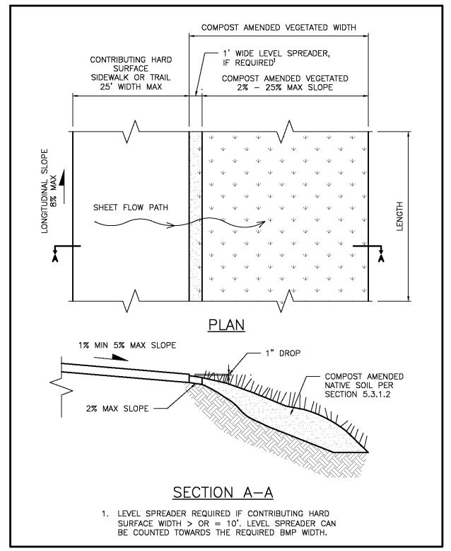
Figure 5.7. Typical Sidewalk/Trail Compost-Amended Strip BMP.
