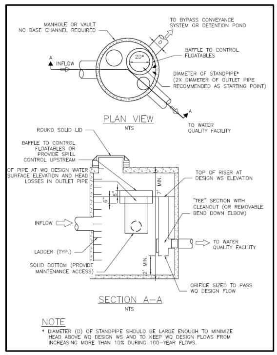
Figure E.6. Flow Splitter Example B.
