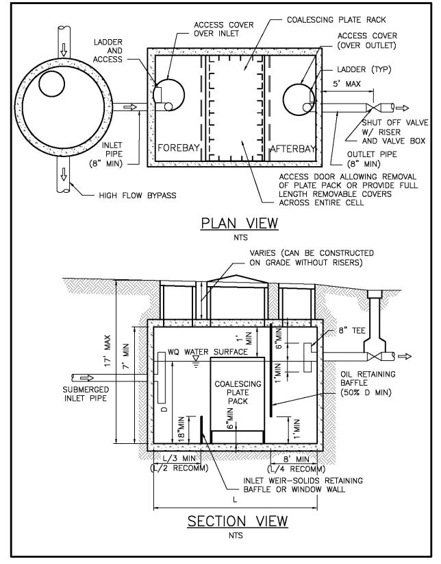
Figure 5.34. Typical Coalescing Plate Separator.
