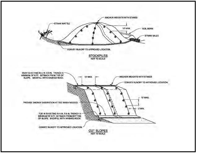
Figure 3. Stockpile Covered with Plastic Sheeting.
