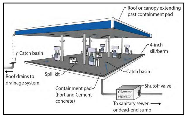
Figure 3. Fueling Island Schematic.
