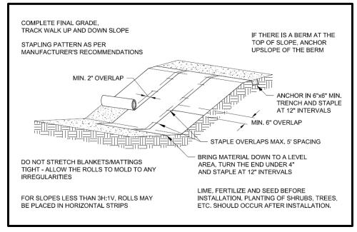
Figure 2a. Mat Installation on Slope.
