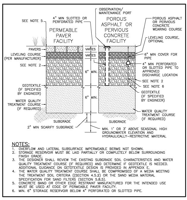
Figure 5.17. Permeable Pavement Facility.
