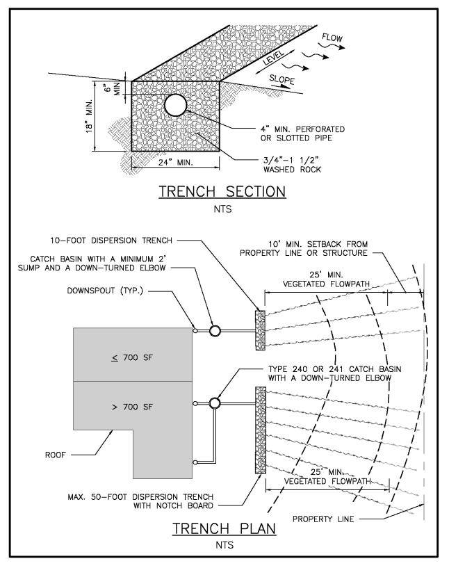
Figure 5.4. Typical Downspout Dispersion Trench.
