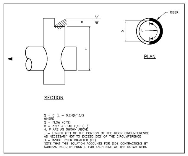
Figure E.3. Rectangular Notch, Sharp-Crested Weir.
