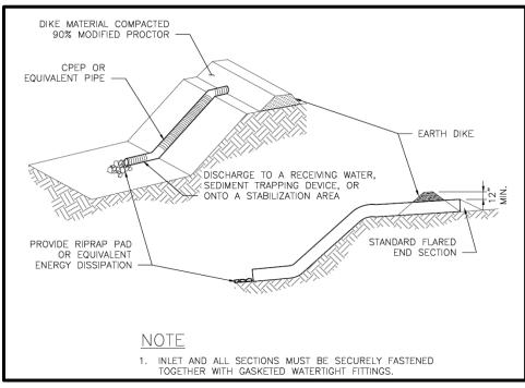
Figure E.8. Pipe Slope Drain Details.
