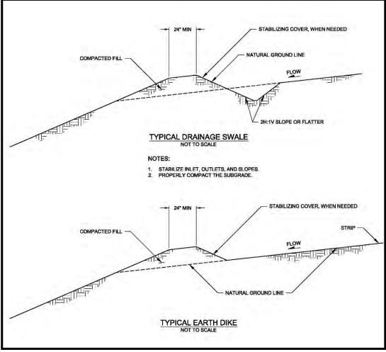
Figure 12. Earth Dike and Drainage Swale.
