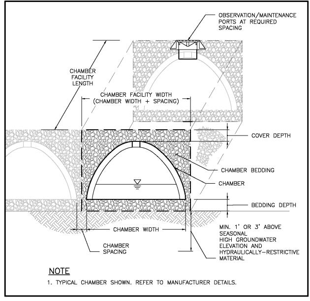
Figure 5.22. Typical Infiltration Chamber/Vault.
