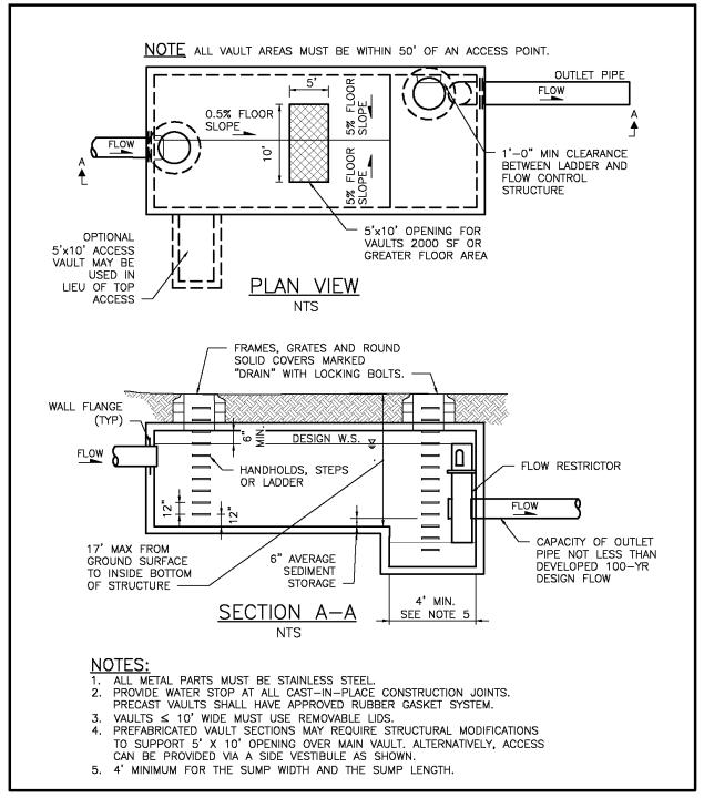
Figure 5.27. Typical Detention Vault.
