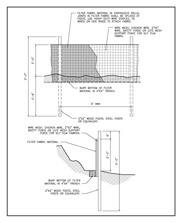
Figure 14. Filter Fence Details.
