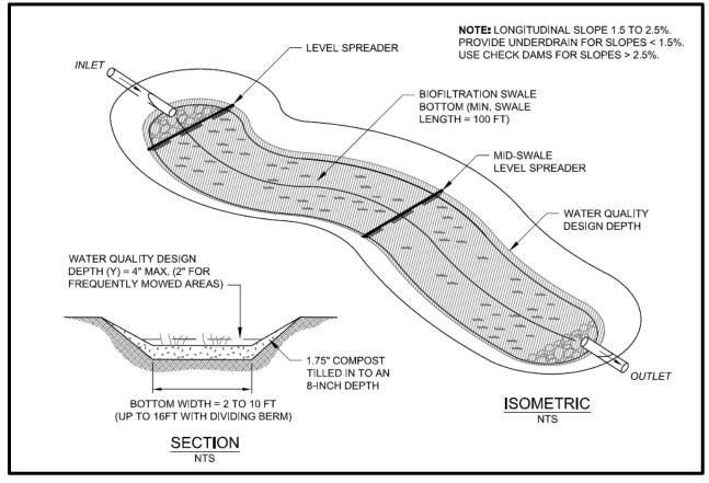
Figure 5.31. Biofiltration Swale Plan and Profile.
