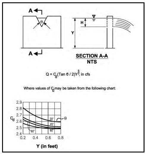
Figure E.2. V-Notch, Sharp-Crested Weir.
