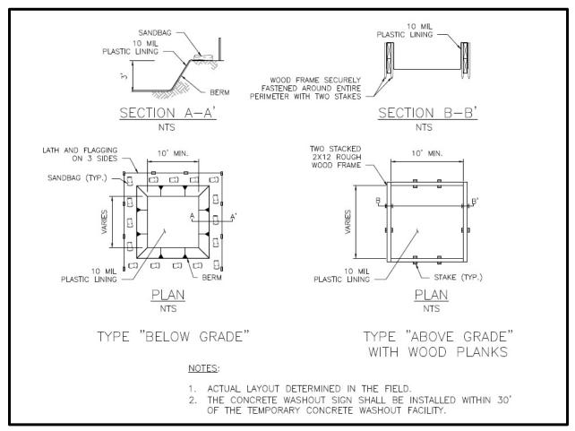
Figure 20. Concrete Washout Facility.
