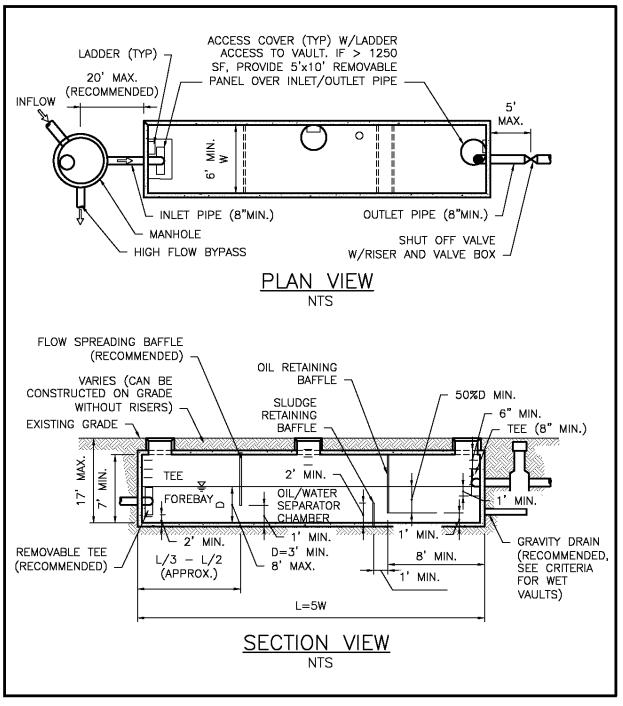
Figure 5.33. Typical API (Baffle Type) Separator.
