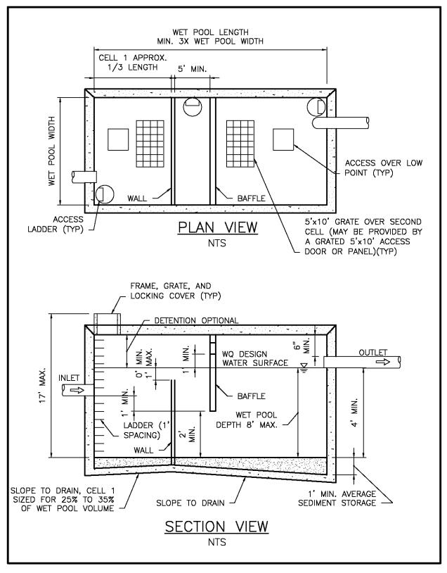
Figure 5.32. Typical Wet Vault.
