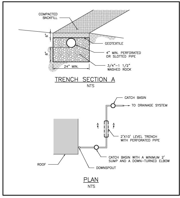
Figure 5.21. Perforated Stub-Out Connection.
