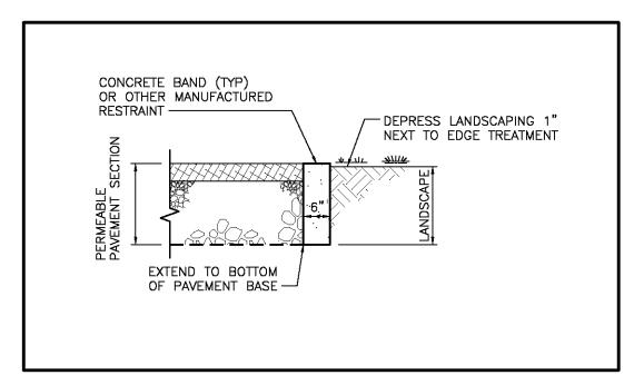
Figure 5.19. Example Permeable Pavement Concrete Edge Treatment.
