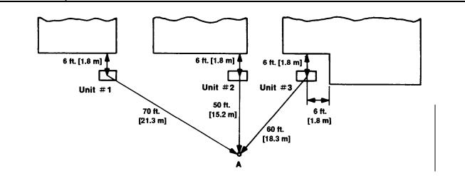
Sound Rating Level of Unit #1 - 68 dB Sound Rating Level of Unit #2 - 68 dB Sound Rating Level of Unit #3 - 72 dB
