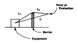
$$\begin{split} L_1 + L_2 &= \text{Distance from equipment} \\ \text{point of evaluation around barrier (Use} \\ \text{minimum } L_1 + L_2 \text{ value.)} \end{split}$$
