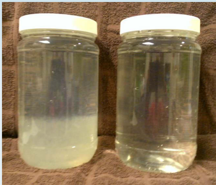
Green Lake alum jar test on 2/20/16 at 82 mg/L (left) and 8.2 mg/L (right)
