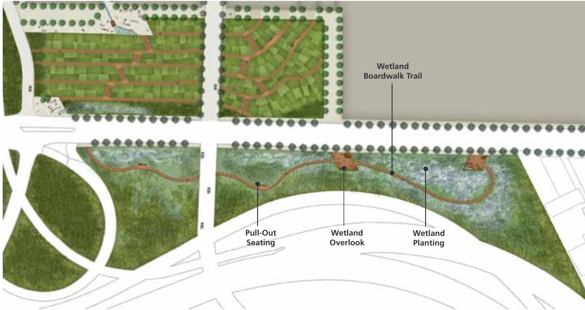
A constructed wetland created to collect the stormwater from the district and provide an amenity for the community
