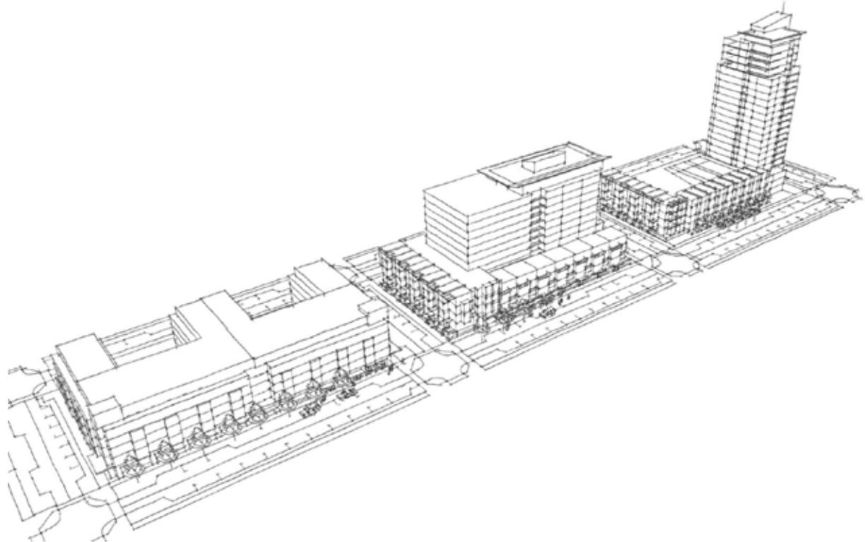
*The illustration above shows three buildings with roughly the same capacity (in floor area) distributed with different heights and massing. This suggests the benefits that taller tower forms can bring in allowing other portions to be lower-scaled.*
