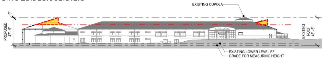
BUILDING HEIGHT - EAST ELEVATION
