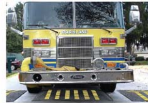
Speed cushions allow for larger vehicles such as fire trucks to pass through unimpeded.
