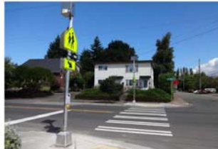
Crossing beacon with push button at a school crosswalk.
