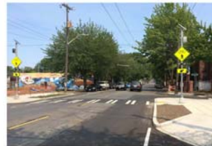
Crossing beacon at neighborhood greenway arterial crossing.
