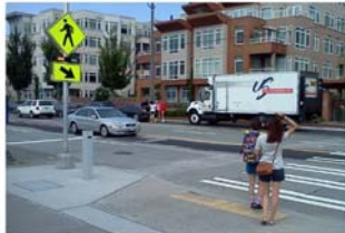
Crossing beacon with passive detection.
