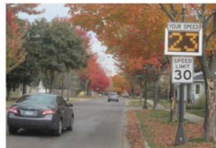
Speed feedback sign displays a driver's speed compared to the speed limit.
