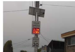
Speed feedback may also flash a "slow down" message.
