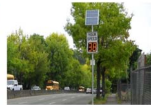
Solar powered speed radar sign.
