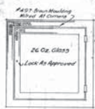
ELEVATION DETAIL OF TELEPHONE BOX IN ENTRANCE VESTIBULE Scale 1/16" = 1'-0"
