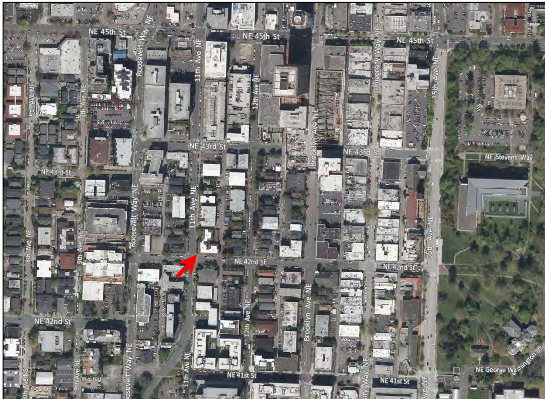
Fig. 2 – Neighborhood aerial photo; subject site indicated by arrow. North is up. The University of Washington campus is visible at right. The series of horizontal bracing bars for the light rail tunnel station excavation are visible one block north of the arrow. (Google Maps 2019)
