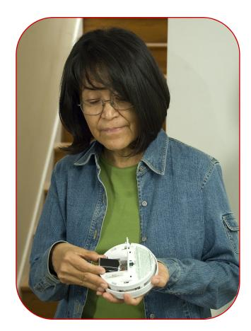
There are many brands of smoke alarms, but two basic types: ionization are quicker to warn about flaming fires and photoelectric are quicker to warn about smoldering fires.
