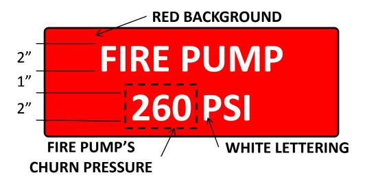
Since your building utilizes a fire pump to provide firefighting water to the sprinkler and standpipe systems, and this fact is not readily observable from the exterior of the building, clear and concise signage is required to assist fire pump operators when connecting fire apparatus with the building during initial operations.
