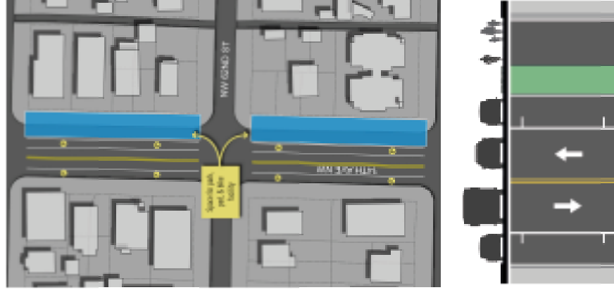
Parking Lane | Travel Lane | Travel Lane | Safety Lane | Access Point for Bike Facility
